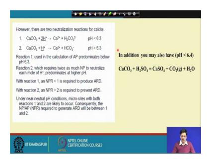
So, this two neutralization reactions; one is calcium carbonate plus 2H is calcium 2 plus H 2 CO3 which happens at an acidic pH; pH is less than 6.3.If that pH is a little higher is more than more than 6.3; then you can accommodate only one hydrogen and will give rise to a bicarbonate ion.
