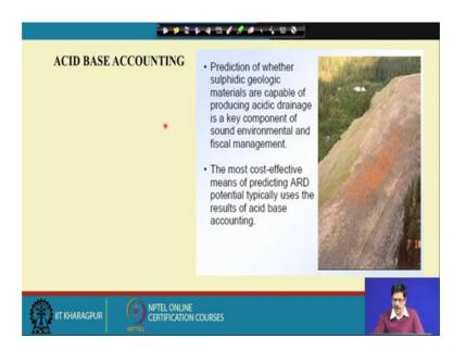
Now, for this kind of environmental impact assessment there are many types of studies which are done. They are the kind of a test which is called as the static tests say acid base accounting is one such kind of static tests. There are kinetic test in which the materials could be studied in the form of putting them in columns and do the experiment in the laboratory.
