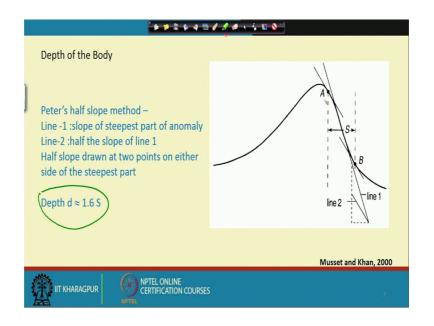
And this gives a very simple formula, very simple idea, as to how to calculate the depth of the ore body, say for example, which is containing the magnetic minerals, here this is the steepest part of the slope of the anomaly, that the curve that you are getting. So, if you draw a tangent here so, that becomes a line 1, and half of that tangent is line 2, and that half tangent line is drawn at points A and B, which are on the either side of the steepest part of the anomaly.
