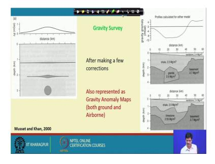
And just let us get some idea about the gravity methods, the way they replied, this is a very simple diagram here, showing that they serve the anomaly that we record here is, because of the presence of a, as a body, which has a much higher density correspond, compared to the surrounding, measured in terms of grams per cc or kg per meter cube, whichever will be more comfortable with a gram per cc kind of a value, which we know that, how the values range in crustal rocks.
