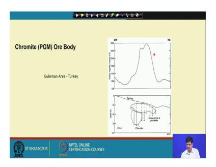
Say for example, there is a Chromite body, and it has been taken one example from of the deposits. So, here this Chromite Body is actually surrounded by a Serpentinite Peridotite on top, and it gives an anomaly which is not that very sharp, but still we could sense the higher magnetic susceptibility of the Chromite Body, compare to the Serpentinized murphy graph.
