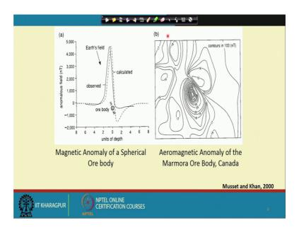
And the situation that can be imagine here, then what we measure essential is an anomalous field, which is measured in nanotesla unit, and this is an Ore body, where this dipole is oriented like this, north and south.
