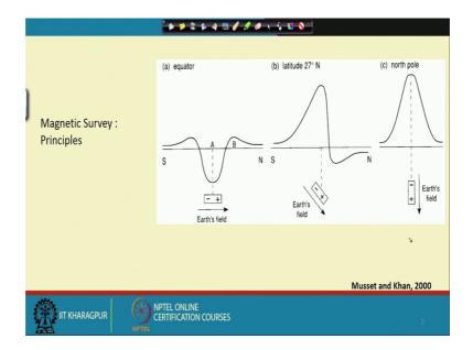
This is an example of a very simple example, which is taken from Musset and Khan 2000. So, here this Magnetic Survey, which is conducted, supposing that our ore body of the material that we are trying to do, trying to measure is a dipole, and it is oriented in respond in parallel to the Earth's field, and this is, the measurement is being done in the equator region.
