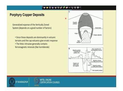
And let us say that, how a Porphyry Copper Deposit will be, will actually show up on a Magnetic anomaly, that is measured on a, on particular this area, where the ore bodies occurring.
