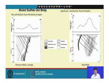
This is an example of a Nickel Sulphide Ore Body, where the, there is no contribution from the Peridotite depth.
