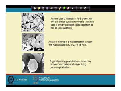
So, this these are some of the photographs, photomicrographs that we have that is that are that I could show you here. Here, it is an example where you see that this is py is for pyrite this is for pyrrhotite is Fe-S.
