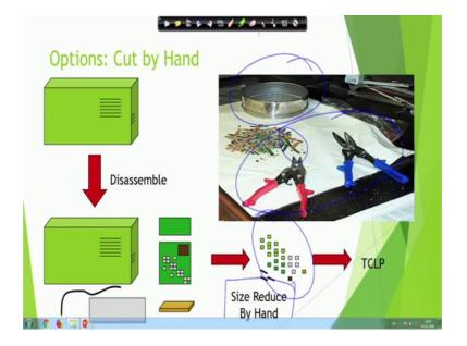
One option we try to do is we cut it by hand option 1 is you try to cut everything by hand it is. So, you have your CPU you disassemble and you have different components in here and. So, disassemble different components and then you try to size reduce my hand up sorry just a minute.
