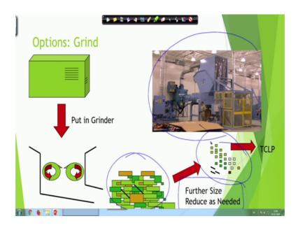
So, grinder will give you some some size reduction then you do the further size reduce by hand as we did in the previous slide and then you get here sample and you work with that sample in terms of the different leaching test. So, that is another option for us to try.
