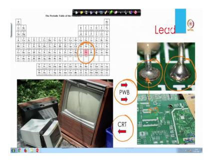
So, as you can see, Lead is the number 1, cause of concern in terms of when we look at the e waste. Lead from the periodic table if you remember, Lead is present; we have the Lead right over there. It is one of the heavy metals. Lead is used in printed wire board that is where we see a lot and CRTs Cathode Ray Tubes. So, this is your when you do the soldering iron this is kind of a zoomed image of a solder on a particular printed wire board.
