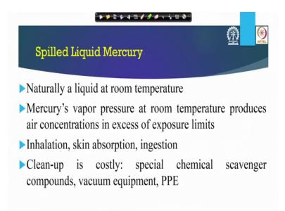
So, there could be Spilled Liquid Mercury naturally a liquid at room temperature. So, it is it access. So, vapor pressure at room temperature produces concentration in excess of exposure limit. So, we will actually, what we will do is there? We will also give you a reading material which talks about a little bit of this basic chemistry stuff.
