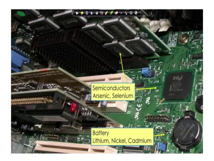
So, again some other like Semiconductors for Arsenic and Selenium, Battery you have the natal Nickel, Cadmium, Lithium; Nickel, Cadmium all those batteries are used. Nickel, Cadmium battery pack is there which is used.
