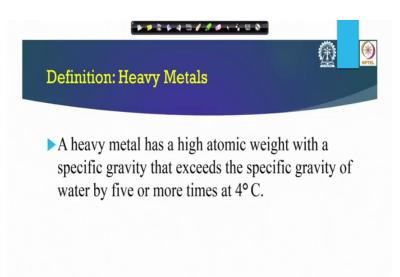
We probably you know heavy metal high atomic weight with a specific gravity of exceeds a specific gravity of water by 5 or more at 4 degrees centigrade. So, some of these just a recap for you.
