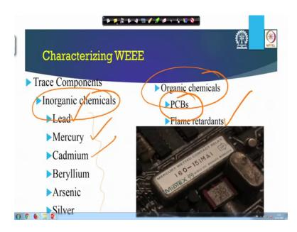
So, in there are different types of, we have a trace components. We have organic chemicals in terms of different types of trace material present. We are looking at Lead, Mercury and. So in terms of the different components as you can see, we have the inorganic chemicals and we have the organic chemicals. So, these are the 2 broad categories of contaminant
