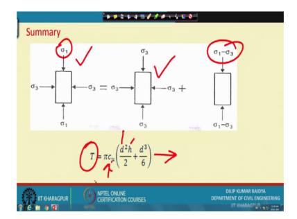
Next thing is; again during direct tri-axial test how happens absolutely apply first the sigma 1 and then this is the final. And we initially apply sigma 3 and later on we apply sigma 1 minus a.
