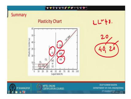
We use plasticity chart that we will find out liquid limit and plastic limit and based on that I do, I find out the plasticity index and other side I put liquid limit and then this is the plasticity standard chart. If this chart actually the if a particular soil is having liquid limit is suppose 30 liquid limit is 40 equal to 40 and your plasticity index suppose 20 pi is equal to 20. Then this 40 and 20 I will put 40 and 20 then 40 s here and 20 is here.
