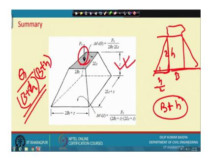
Generally we consider the 1 vertical 2 horizontal sorry 2 vertical 1 horizontal; that means, if you go down this much then you will horizontally will be half of that so, if this is this height is h then it will be this such spreading will be h by 2. So, that means, if the footing is here then I can assume the footing is widened at this depth equal to this side h by 2 and this side also h by 2. So, ultimately footing which was originally B then it will be at that depth B plus h.
