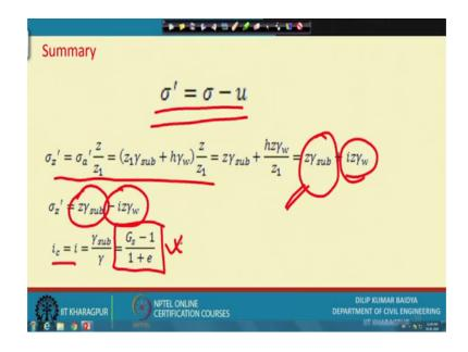
Then this is again same thing I have mentioned and this is the static conditions the effective stress is total stress minus u and when water flow through the soil again the effective stress is not be like this.
