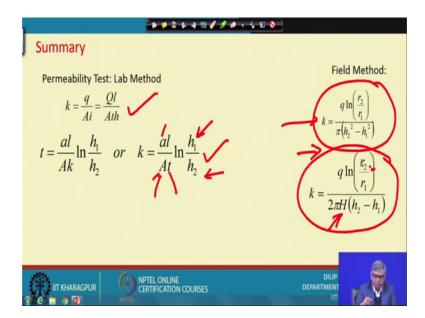
So, next is suppose there is a permeability also another important characteristics of soil. So, you need to know the value of permeability available because it is a important properties for soil. And soil permeability can be determined in different ways either in lab or in field.
