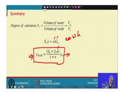
So, next is; the next thing was that degree of saturation on porosity, void ratio at degree of saturation and certain relationship between them like degree of saturation then porosity then water content and specific gravity. This is also a very standard relationship and the soil is fully saturated then e equal to w into G because fully saturated means at w equal to we equal to actually S equal to 1.
