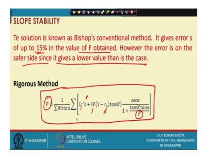
So, the solution given is known as Bishops conventional method and it gives error up to 15 percent in the value of F obtained. So, and 15 percent error in the value of F; however, the error is on the safer side, since it gives a lower value of a value than it is actual.
