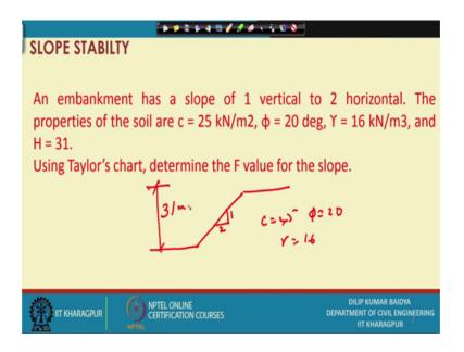
So, this problem is something like this and embankment has a slope of 1 vertical to 2 horizontal and the prop properties of the soil c equal to 25 and phi is 20 degrees and gamma equal to 16 kilo Newton per meter cube and H equal to 31; that means, your slope 1 vertical 1 vertical 2 horizontal.
