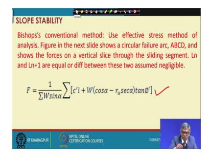
So, now next thing is that a rigorous method and in the rigorous method actually first introduced by Bishop and Bishop consider conventional method actually use effective stress method and figured and the next slide that is the figure actually one particular slice should be shown.
