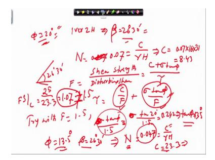
So, I will not do that, what I will do I will do for phi equal to 20 degrees. And slope angle actually 1 vertical, 1 vertical, 2 horizontal corresponding to it gives you alpha equal to 26 degrees 30 minutes so; that means, the slope at the slope 26 degrees 30 minutes.
