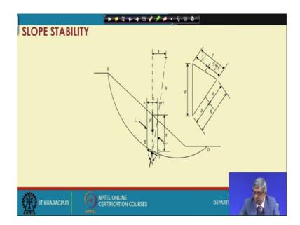
So, if you so, the better I will go to the next slide so, this is the slope suppose this is the slope and then on this slope there is a slice taken suppose one slice is taken here and on that on that slice what are the forces acting? This self weight of the slice it is acting. Then from the left side that will be force acting from the left side and from the right side there will be some force acting and there will be tangential force acting there is a normal force acting.
