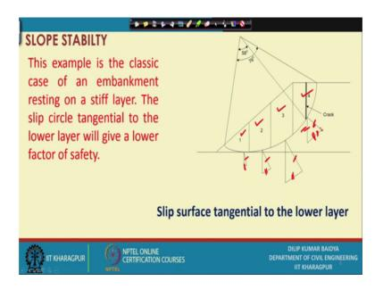
So, next slide so, this is the one of first I will the embankment resting on a stiff layer and the slip circle tangential to the lower layer will give you a lower factor of safety so; that means, finally, we will show you that. So, we are assuming the first one it is the given like that and we have already explained that when this type of problem we solve and typically we need to divide into number of slices.
