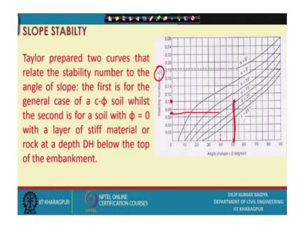
One chart is given; Taylor prepared two curves that relate the stability number to the angle of slope. The first is for the general case of a C phi soil while the second are this is the phi equal to 0 and you can see this is the chart given and either you can do two ways. Generally your phi of the soil is required, it is generally will be known and if it is known and phi and C then you have to what is the slope angle you can provide.
