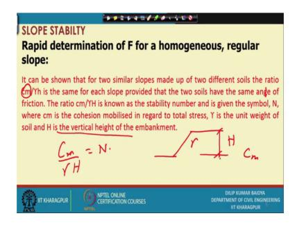
And for these this is actually basically graphical procedure you have to do lot of graphical work and finally, after doing so many assumed slip surface we will get the critical factor of safety and then corresponding to critical factor of safety we will be the actual slip surface, that is one way can be done.
