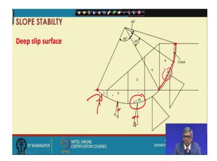
And in these you can see now the initially we are not taking tension crack. So, I am taking from here to here and this angle was a total angle was 85 plus 45.
