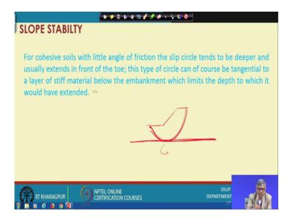
And next to next slide and for cohesive soil with little angle of friction the slip circle tends to be deeper; that means, if this is a slope here and there here. So, generally it will be something like this we go deeper usually extends in front of the toe; that means, it will go the beyond that.
