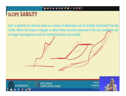
And this method such a method or can only be used as a means of obtaining a set of sensibly positioned trial slip surface. When the slope is irregular or when there are pore pressure in the soil conditions are no longer homogeneous and the method becomes less reliable.
