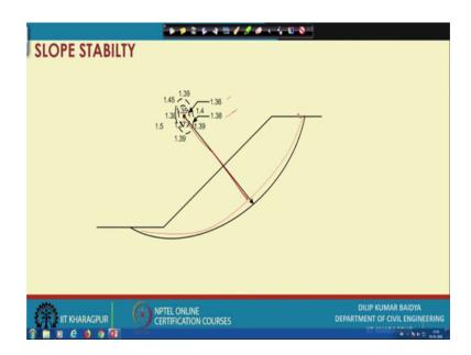
You can see here so, this is the one. So, you can see that suppose one point we have got initially suppose of the number of points and finally, we have got a contour of 1.39, contour of 1.36 sorry contour of 1.38, 1.36 and 1.35 maybe somewhere here and value maybe is there 1.39, 1.45, 1.5 there are a number of values are there.
