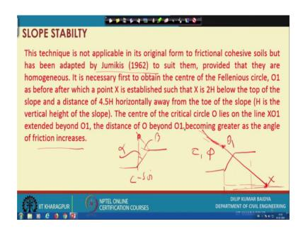
So, this technique is not applicable in it is original form to the frictional cohesive soil; that means, where soil is have processing both c and phi ah; that means, what we have we have done when they c soil you are getting by drawing a line from here and drawing a line from here this is the or c soil ok. So, this is beta and this is alpha and given by the Fellenius, but when you this is applicable for that one.
