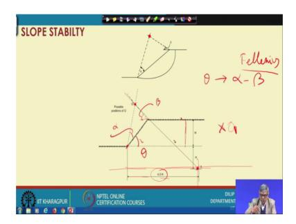
This is the failure surface sorry this is the slope and you can see you can locate 2 and locate the end of the slope, this two point. And from this point you draw a line with the sloping surface at an angle alpha this is the line with angle alpha. And again you can draw another line with angle with horizontal passing through the end of the circle with angle beta and draw another line.
