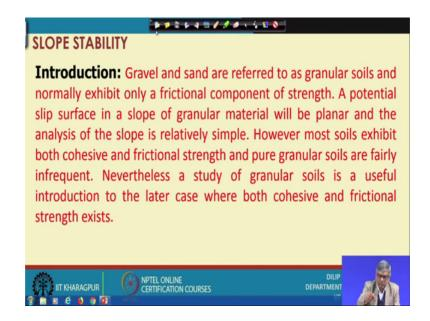
And under that is a gravel and sand one type of soil which will have will be named as granular soil and it has only a frictional component; that means, when you calculate the strength then it has only tan phi which gives you slip is constant. And potential slip surface; that means, if you make a sand a slope with sand then your slope will be granular, so material will be planar; that means, it will not be a curves.
