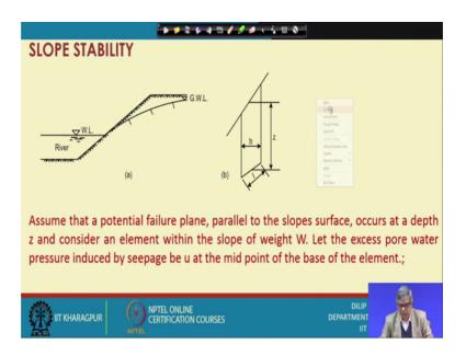
First of all I will show how doing this is the slope suppose and when water table is here the natural fleetic line or a ground vertical initially will be like this only ok. So, it will be like this and so now if I on this slope if I consider a mass like previously then it will have water pressure. So, in this there are number of things I have shown I have taken width of
