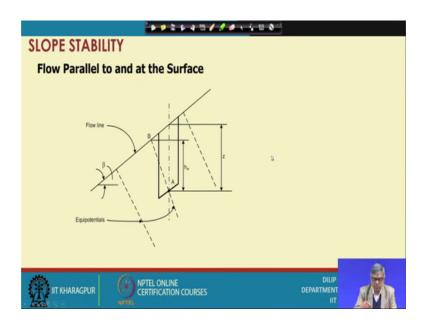
And now let us see one more a thing when the flow is taking place parallel to the slope of the so this is the one. So, earlier we have considered a theoretic surface initially you have considered a frenetic surface which was a curved one. And now that we are considering the flow is actually parallel to this along these and parallel to this, so, flow is taking place in this direction.
