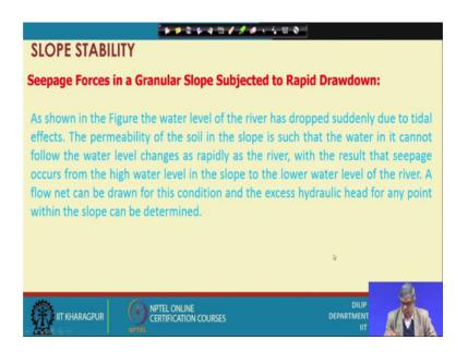
This is actually the seepage force in a granular slope subjected to rapid drawdown; that means, you are now considering introducing seepage, and you can see in the next figure I will go let me go to the next figure.
