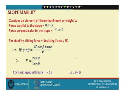
And based on these force polygon what you can do? We can we can see we can as I have mentioned we have taken the element on the embankment, and W is the force weight and the force parallel to the slope will be W sin beta which is shown as t, and force perpendicular to the slope will be W cos beta that is angular. If the slope is this angle is beta then this slope that this component and this component acknowledge W sin beta and another is W cos beta.
