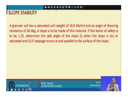
Next one there will be problem given here a granular soil has a saturated unit weight equal to 18 kilo Newton per meter cube, and angle of shearing resistance equal to 30 degree, a slope is to be made of this material. If the factor of safety is to be 1.25, determine the safe angle of the slope, when the slope is dry or submerged and the seepage occurs.
