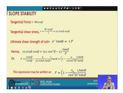
Similarly if I shear strength you have to calculate. So, you can go back to this you can see the tangential force is W sin beta and tangential shear stress again the load by area and I again to be substituted then it will be gamma z sin beta cos beta ok. And so this is the tangential shear stress.
