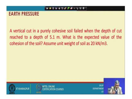
You can see a vertical cut in a purely cohesive soil failed when the depth of cut reached to a depth of 5 meter, 5.1 meter. What is the expected value of the cohesion of the soil? So a pure cohesion cohesive soil is mentioned and excavation is going on and suddenly when reduced to 5.1 meter it failed.
