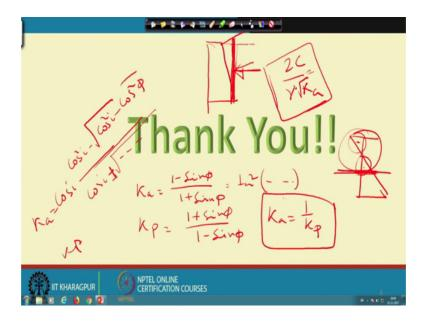
And K a also will be equal to 1 plus sin phi by 1 minus sin phi. So, from there we can see that K a equal to 1 by K p. So, this is also another point to be remembered and when there is slopping surface then the K a little modified K a equal to cos i, and then you have you have cos i minus under root cos square i minus cos square phi divided by cos cos i minus under root this is plus.
