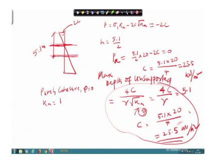
You know that pressure diagram is something like this ok. So, purely cohesive phi equal to 0 so; that means, your K a become 1, that is one thing. And at this point what will be the value actually this is actually you have p equal to sigma 1 K a minus 2 C root K a, so this is the one.
