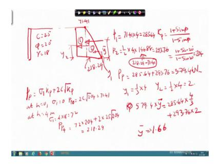
And you can see the wall height was how much I think 4 meter height. So, wall was of 4 meter height. So, this is 4 meter, and it has level and C equal to 25, phi equal to 20 and gamma equal to 18, so it will have since we are going to we are going to apply as the passive case. So, I have to find out now K p K p equal to what 1 plus sin phi by 1 minus sin phi.
