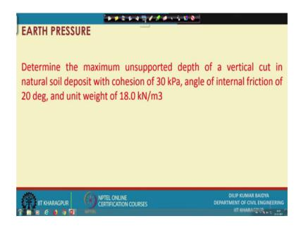
This is suppose determine the maximum unsupported depth of a vertical cut in natural soil deposit with cohesion of 30 kPa, angle of internal friction of 20 degrees, and unit weight of 18 kilo Newton.
