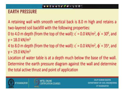
So, let me take problem number 1. The problem number 1 is like this; a retaining wall with smooth vertical back is 8 meter high and retaining a two layered soil backfill with the following properties. so 0 to 4 meter depth from the top depth, from the top of the wall c is 0 phi 30 degrees and gamma 18. So, this is a cohesion less soil, basically, first layer, second layer 4 to 8 meter depth from the top of the wall also again c 0, phi 35
