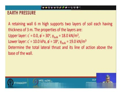
So, let me go to the second application, second application somehow is a two layer soil again top layer is you can say is a phi soil and bottom layer is c phi soil, retaining wall six meter high suppose two layers of soil each having thickness of 3 meter the properties
