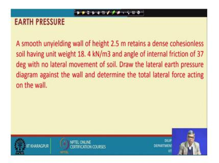
So, first problem used like this smooth unyielding wall of height 2.5 meter return retains a dense cohesionless soil having unit weight 18.4 kilo meter per cube and angle of internal friction of 37 degrees with no lateral movement of soil. Draw the lateral earth pressure diagram against the wall and determine the total lateral force acting on the wall.
