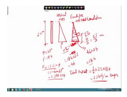
So, here we know K naught equal to 1 minus sin phi. So, 1 minus sin 37 degrees that gives you 0.398 or equivalent to 0.4, I can take. So, if I do intensity of vertical stress over depth. So, if I do intensity of vertical stress over depth, this will be gamma times gamma times h. So, it will be equal to 18.4 multiplied by 2.5. So, this will be your 18; that will be 46 and then, if I want to this is actually vertical stress.
