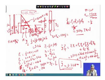
So, you have K a equal to 1 minus sin 30 divided by 1 plus sin 30. So, that gives you 1 by 3, and then you can find out gamma equal to 18. So, suppose I can take a wall somewhere here, I take a wall somewhere here and this height is 5 meter and water table was somewhere here, that is 2 meter and the total unit rate above and below the water table is can be taken as same. So, unit rate is given 18 kilo Newton per meter cube gamma equal to 18 kilo Newton kilo Newton per meter cube it is given.
