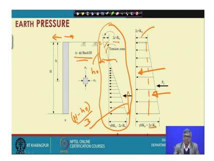
Next let us see the once again together active and passive how is the pressure diagram I will show again. So, you can see here the soil cohesive backfill and with having c and phi and sigma 1 and sigma 3 like this, because of the wall movement in this direction or these direction. So, moves these direction this is the active case and your pressure diagram will be something like this, at this point 2 c root k a at this point gamma is k minus 2 c root k a.
