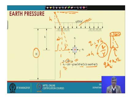
Next you can see now there is one more part I have only considered so, far the only the backfill, sometime on the backfill also over the backfill there may be priorities of equipment may be there, for some work, or some other reason some loading may be there. So, if there is a cost and loading over the surcharge in the form of surcharge is there, how to find out the pressure diagram.
