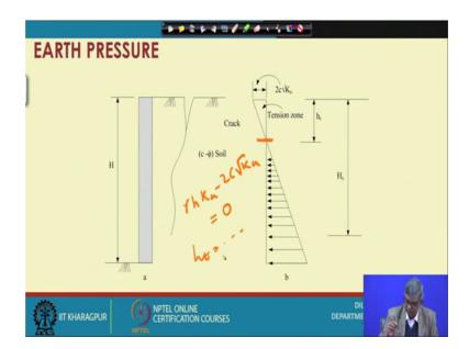
Now, you can see as I have mentioned that when it is active case, you have you will have negative pressure negative lateral pressure negative lateral pressure means, what it is tension when there is a tension means while actually will have cracks. So, this is the way it can crack actually for c phi soil. So, we can find out what is the depth at which tension will create.
