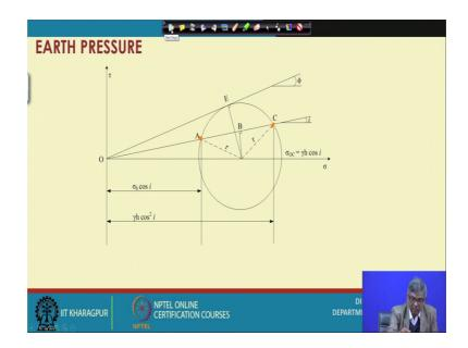
Now, that we are talking about the Mohrs circle this is the Mohr circle a normal case, horizontal when it is a horizontal backfill, this is the Mohrs circle and now if the there is a sloping surface is there at a angle I and you can draw a line through the origin to at a angle I and then it will be intersect this 2 point on the circle then we will be representing actually vertical stress and lateral stress.
