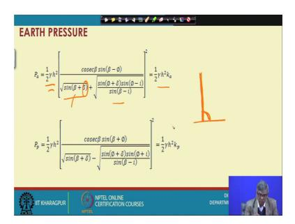
We can see that we will get a expression for Pa equal to half gamma h square equal to cosec beta sin beta minus phi under root these and these whole square equal to half gamma h square Ka. So, now, what is delta that is angle between the because of the friction the back fill and the wall because of that that delta and beta is the angle from the back fill inclination.
