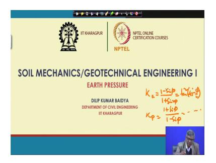
And this active earth pressure coefficient and passive earth pressure coefficient, they are known that is Ka equal to 1 minus sin phi by 1 plus sin phi or equal to tan square 45 degree minus phi by 2 and similarly K p equal to 1 plus sin phi by 1 minus sin phi and corresponding this value also similar. So, these are the things already we have know we have discussed and how to find out the thrust behind the wall some we have given.
