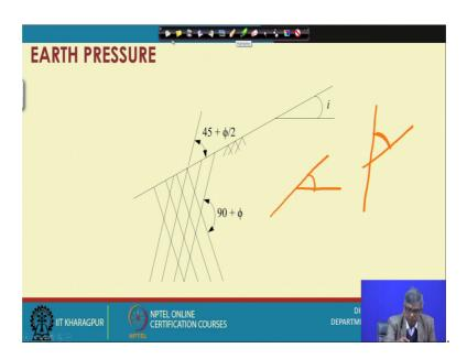
And it is of course, failure planes failure planes will be for the such thing the same 45 degree plus phi by 2 with respect to this.
