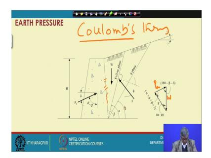
We assume Rankine theory this is coulomb theory. Actually in Rankines theory before. So, for you have discussed Rankines theory, Rankines theory actually there are set of assumptions assumption are wall is vertical and there is no friction between the wall and the backfill and level backfill all those things are there, but coulomb theory is very much general; that means, why very much general.
