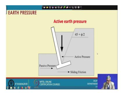
So, this is actually active earth pressure now what was that is a shown I general this is our active and. So, when this active earth pressure happened this way is actually from the horizontal this line, this failure plane makes an angle 45 degree plus phi by 2 where phi is the angle of internal friction of the soil. And so, this will be there and. So, based on that I can if I can now draw a Mohr circle you can see if you draw Mohr circle for active case.
