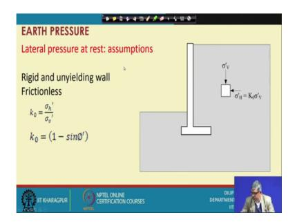
When active case when active case wall moves out whereas, in passive case wall move seen as I have told you this is a wall and this is a back fill. So, in the wall these is an active and wall is this towards back fill that is passive. And shear stress on failure plane reduces; that means, active case since you can see the wall when it is a no movement whatever pressure will be there it wall moves, that mean it will reducing pressure will be reducing over time.
