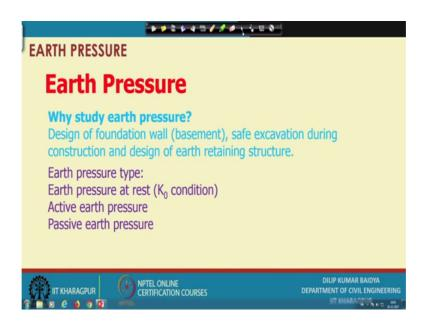
You can see earth pressure why study earth pressure ok. So, this is basically design of foundation wall basement safe excavation during construction and design of earth retaining wall all for those case actually you need to know earth pressure.
