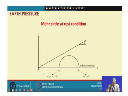
And you can see if I want to see the Mohr circle corresponding to the at rest condition you can see that if the soil as a friction angle equal to phi then this will be the your failure envelope ok. And your you are at rest condition sigma v suppose this one and sigma h suppose this one or sigma h or sigma h h or x h can be there it is z or v either or a.
