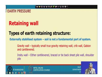
The types of earth retaining wall ok; So, this is the major or classification can be done externally stabilized system; that means what, soil is not a fundamental part of the system.
