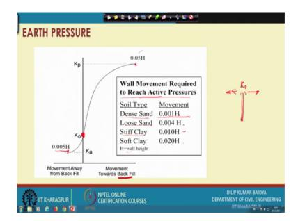
Now, you can see to get earth pressure as I have told you that wall moves. So, this is wall and suppose wall moves in this direction ok. How much movement is generally is expected before failure? Even movement is more than that then you consider is fail.
