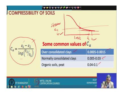
You can see. So, we have shown (Refer Time: 25:43) versus strain versus log time. And we have a curve something like this. So, somewhere maybe the end of primary consolidation and it will keep the loading here continuously, then you get a curve like this. So, from here this is suppose end of primary consolidation ok. And now suppose I extend this one, a straight portion I extend.
