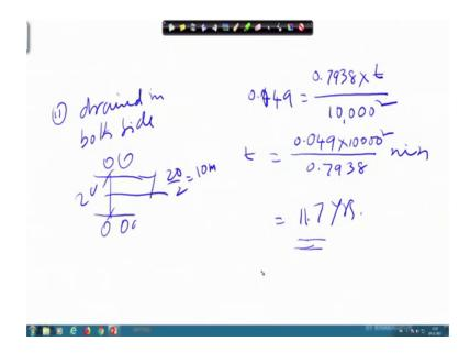
But if I want to do next one drained in both side. So, drained in both side that means, the same one draining here, draining here, and this is 20 meter, so your edge become 20 by 2 actually 10 meter. So, here also I can do 0.49, 0.049 equal to C v actually 0.7938 into t is unknown and H is here 10,000 square. So, it gives you t equal to 0.049 into 10,000 multiplied 10,000 square divided by 0.7938, this will be in minute.
