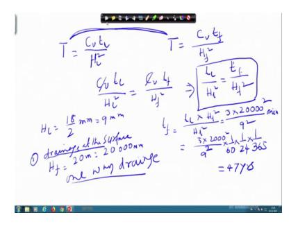
So, I will take the first one by first method that is your you can see as I have told you the laboratory sample suppose I will say this is T for laboratory and that will be equal to C v t by H square. And for field also similarly suppose this is also T equal to C v t, so this is about t lab L suppose and this is suppose t field and this is suppose H field square and H lab square.
