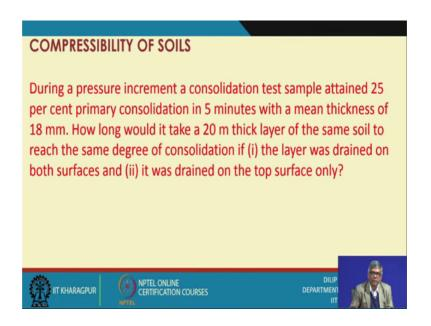
So, I will start with the first one. This is the problem description. During a pressure increment a consolidation test sample attained 25 percent primary consolidation in 5 minutes with a mean thickness of 18 millimeter. How long would it take a 20-meter thick
