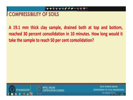
So, next is next problem you can see a 19 milli 19.1 millimeter thick clay sample 19 drain both at top and bottom, reached 30 percent consolidation in 10 minutes. How long would it take the sample to reach 50 percent consolidation ok? So, this is the one question is there. The sample thickness is given 19.1 and drained both side, it is also mentioned and 30 percent consolidation reached in 10 minutes.
