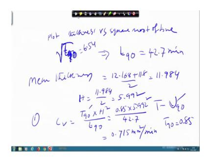
So, let me see how to do this you can see we have to plot first we have to plot thickness versus thickness versus square root square root of time that will get. And from there will from there corresponding to (Refer Time: 28:01) root t 90 will get at t 50 we will sorry not t 50 we will get t 90 here. We will get root t 90, root t 90 we will get from here. And from there we will get t t 90 actually.
