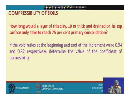
And then after that you can see how long would a layer of this clay, 10 meter thick and drained on its top surface only, take two reach 75 percent primary consolidation? And then; if the void ratios at the beginning and end of the increment where 0.94 and 0.82 respectively, determine the value of the coefficient of permeability.
