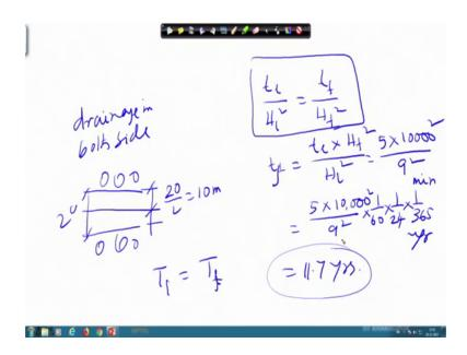
Now, I will say drainage in both side in both side that means in the clay layer is here and this is draining layer this is also draining layer and this is 20. So, your drainage path will
