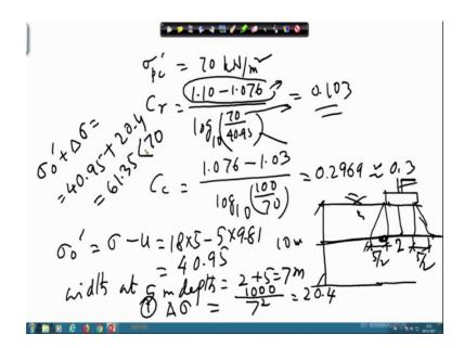
And C r can be calculated which will be equal to can see two points pressure is given and void ratio is given. So, deltas void ratio or delta e 1.10 minus 1.076 and their corresponding pressure is log 10 base 70 by 70 by 40.95. Actually at 70 pressure we have this void ratio around 40 pressure this is a void ratio. So, because of this two pressure void ratio changes. So, this is delta e divided by log P 2 by P 1. So, this gives you C r that value if you calculated comes actually 0.103.
