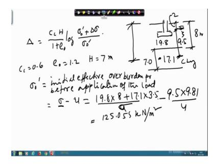
Sorry; and from here this is 7 meter and this is 8 meter and water table is at 2 meter from here, this is 2 meter. So, this is water table and the soil properties given here 19.8 here it is given 19.8 here it is given 17.1. So, this is the information we have. So, what other information we have? As we have decided we will be using the a formula delta equal to C c into H by 1 plus e naught log sigma naught dash plus delta sigma divided by sigma naught dash.
