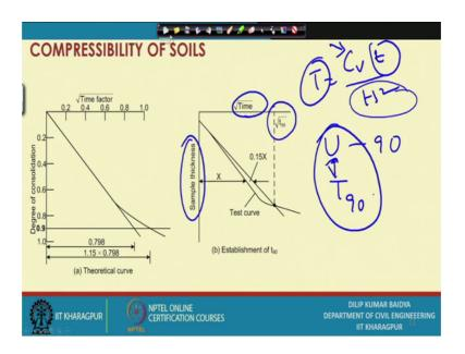
So, from here actually from this plot we can read. So, we have got intestine. So, T 90 we will get from that test here and U 90, then corresponding T 90 I can get from the relationship between T and U. So, once you get T equal to C v T by H square. So, when you carry out contest H is known T we are getting from here and T you are getting from
