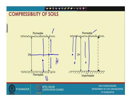
So, your drainage path will be H and this is schematically shown in this; you can see this is permeable and this is also permeable. So, water particle from here maximum distance travelled, if it goes whether it goes this way or this way that distance is still H, but if the water particle is here it will never go this way, because before that if it goes there it will be faster. So, they will try to release faster, because it is under pressure.
