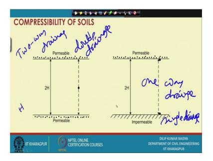
So, that is the thing that, these two symmetrical diagram two ways drainage or it is all this called double drainage. And this is one way drainage or sometimes called single drainage ok. So, double drainage actually there are H will become half the thickness of the layer, when single drainage that it will be like thickness of the layer itself will be the H.
