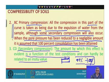
Primary compression that is, whatever consolidation mechanism we have explain. All the compression in this part of the curve is taken as being due to the expulsion of water from the sample, although some secondary compression will also occur.
