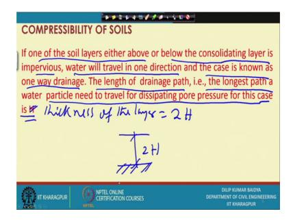
So, this is same thing repeated here, whatever I had just told if one of the soil layers either above or below the consolidated layer consolidating layer is impervious water will travel in one direction and the case is known as one way drainage.
