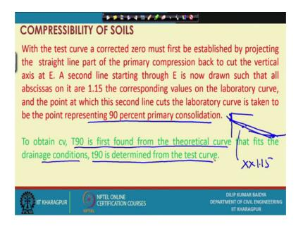
So, once again whatever I have mentioned and just repeat with the test curve we corrected zero must be must first be established by projecting the straight line part of this so; that means, if you have the curve like this. So, you extend this straight portion we will gets though the curve started here, but you can yeah consider start of constellation here line of the primary compression back to cut the vertical axis at E. So; that means, this is the point E.
