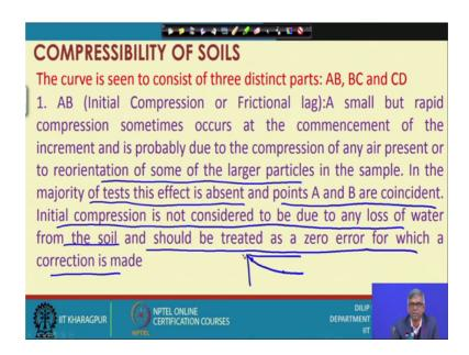
So, we will explain one by one what are those you can see the car was seen to consist of three distinct part AB, BC and CD and AB is the initial compression or frictional lag. So, because of this it is a it is at a ring sample will be prepared and it will load and then compression will be observed.
