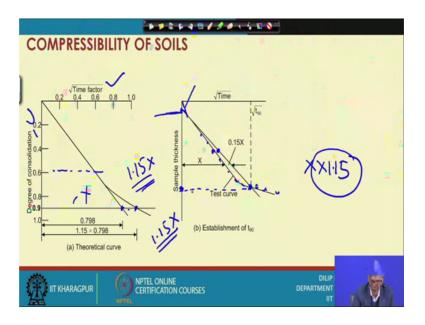
This is the one observation is given; initially the root time factor versus degree of consolidation U plotted like this, and up to 60 percent is perfect straight line and then started deviating from the straight line.
