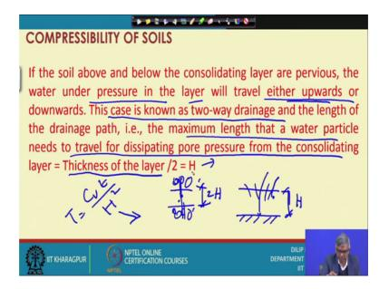
At the only one side is rock and one side is pervious soil. So, water will flow in to one direction sometime there will be the layer this side this side both side actually pervious soil. So, pro will be in the both direction. So, accordingly whatever equation we have used T equal to Cv t by H square, this H actually the longest distance the water particle to move to dissipate the pore pressure.
