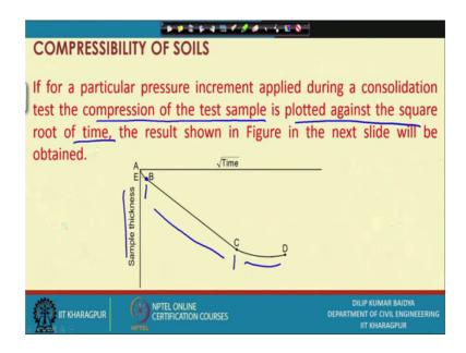
Now, T versus U you know now T versus sample thickness observation it is seen that for a particular pressure intimate applied during a consolidation test. The compression of the test sample is plotted against the square root of time square root of time versus sample thickness, if it is plotted, then we get a curve like this initially a small curve portion.
