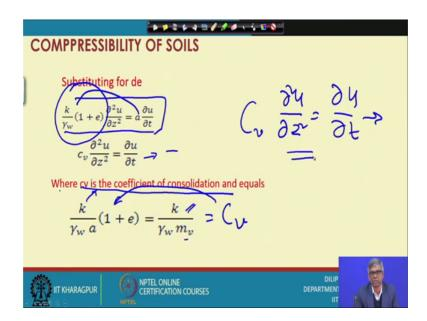
Now you substitute those. Then it become in this form. The equation will come to this form k gamma w 1 plus e del 2 u del z square a del u del t or C v into del u del 2 u del z square equal to del u del t. And now we are taking this one cv is defined, a coefficient of consolidation which will be k gamma w a into 1 plus e equal to k by gamma w. So, C v that is C v. C v equal to k by gamma w m v or C v equal to k by gamma w a k into 1 plus e by gamma w into a.
