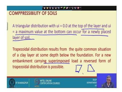
And similarly it a triangular distribution with ui equal to 0 that is newly deposited because they are actually since is a loose and immediately after deposition there if there is a pore pressure development immediately it will dissipated. So, at the top of the layer and ui equal to a maximum value at the bottom can occur for newly newly placed layer of soil. So, because of this reason already I have explained.
