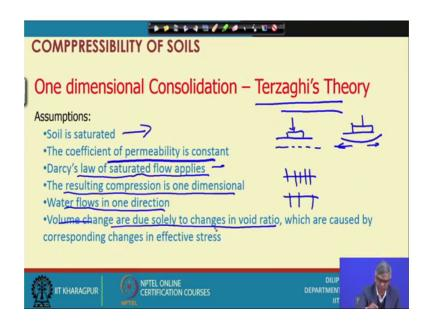
Now, the consolidation settlement that will be theory developed by Terzaghi's firs that is actually one dimensional consolidation theory; later on three dimensional consolidation theory also developed. But we will concentrate right now on one dimensional consolidation theory proposed by Terzaghi. And for any theory you know that we have we need to have certain assumption and if you deviate from the assumption then this will not be applicable.
