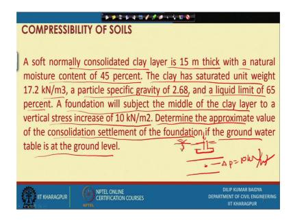
As I have mentioned that very to illustrate the appeal your problem a equation what you have used there is a simple problem we have taken here you can see the problem you saw normally consolidated clay is 15 millimeter thick, with a natural moisture content of 45 percent, the clay has saturated unit weight of this a particle specific gravity 2.68 and in liquid limit of this is 65 percent.
