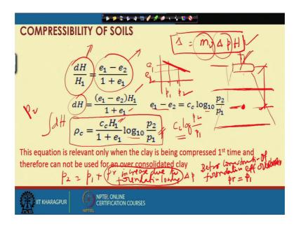
And you can see now observing this e versus log p curve this is a straight line and then you can utilize that to find out the compression we have already developed we have shown one calculation for how to find out that the total consolidation settlement, delta
