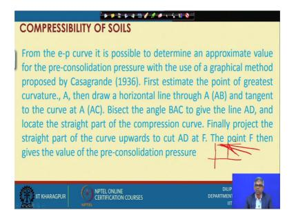
And from the e-p curve it is possible to determine an approximate value for the pre consolidation pressure.
