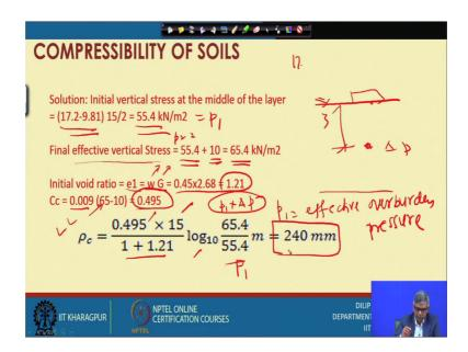
So, based on that let us see the calculation. So, the clay layer thickness was something 15 meter. So, 15 meter thick layer and water table is here and. So, you can see the because of this foundation at the middle actually del p is given, but what you have to find out p 1, p 1 is nothing, but effective overburden pressure ok; So, effective overburden pressure.
