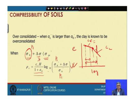
As I have mentioned before that e versus log p curve we generally take if this way this is e and this is log p and this is cr and this is Cc this is actually p consolidation pressure this is the way we take.
