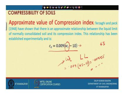
So, before going to that problem let me as I have mentioned that Cc is the slope of the e log p curve, but I also I have mentioned that there are several methods available to find out Cc one such method is given by Terzaghi actually Cc equal to 0.009 into liquid limit minus 10.
