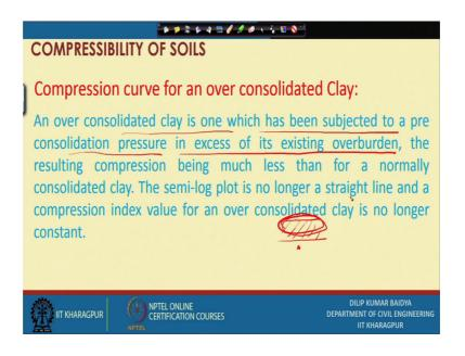
This is so, how and how will be what is the over consolidated soil and how will be the compression curve of a over consolidated clay and let me first define what is the over consolidated clay. And over consolidated clay is one which has been subjected to a pre consolidation pressure in excess of its existing overburden; that means, suppose at a particular depth at a at or at any point say all at any point.
