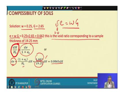
There are two three methods actually can do and one method I will just first explained that is actually from the end actually can start and solution is since at the end of the consolidation where after removal of the low quantity it is fully expanded at that condition also soil will be saturated. And water content was measured 20 point 25 percent and G was 2.65.
