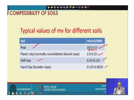
So, this is one way to find out the compression that is called mv approach; that means, by using coefficient of volume compressibility one can find out the comp compression of the soil or settlement of the soil consolidation settlement of the soil.
