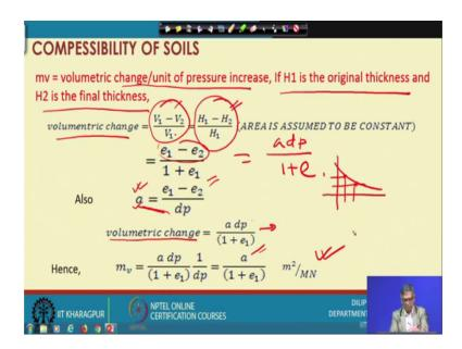
And then mv defined as a volumetric change per unit pressure sorry volumetric change; volumetric change per unit pressure that is in mv H 1 is the original thickness and H 2 is the final thickness the volumetric change this way you can write also I can write it in this way because area if it is constant.
