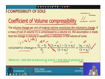
Now, if want to estimate the amount of compression then we use a term that is coefficient of volume compressibility. And this is; what is the definition actually the volume change per unit of original volume constitute the volume volumetric change ok.
