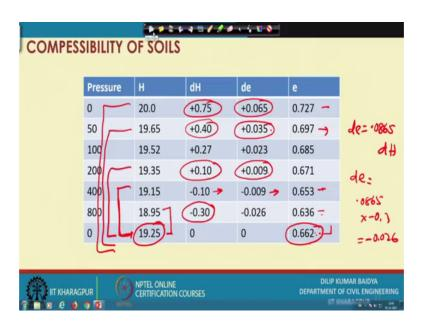
19 point 19.25; 19.25 and thickness and void ratio this one and we have got d equal to 0.0865 de equal to 0.0865 dH. So, we know this is the thickness and this is the corresponding void ratio and we have got change in void ratio in terms of thickness we have got this.
