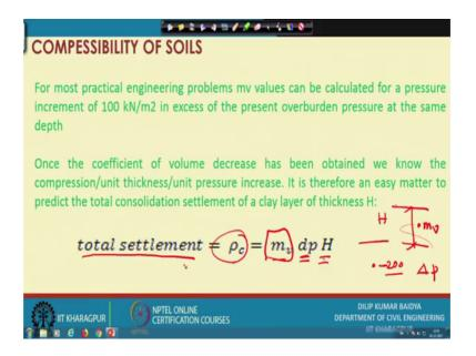
And for most soil most practical engineering problem mv values can be calculated for pressure increment; 100 kilo Newton per meter square in excess of the present overburden pressure. Suppose; that means, in a soil at point what is the effective overburden pressure at present above more than 100 in excess; that means, if it is 200.
