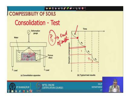
And once a test is called odometer test and odometer test if I see this is the type of sample we keep here the sample is here and this is the stone at top and bottom. And this is actually odometer actually where we put the sample and this sample entire sample will be immerse in water.
