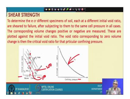
You can see here that we can see at this point, this point actually no volume change and if it is a positive volume increase this side and volume decrease this side if I plot and this side is initial void ratio. Suppose I choose a initial void ratio very small and then I apply confining pressure certain value of confining pressure and then I will see the volume
