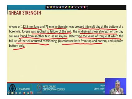
Next I can give you one example of this the problem is a vane of 112 millimetre long and seventy millimetre diameter was pressed in soft clay at the bottom of a borehole. Torque was applied to failure of the soil. The undrained shear strength of the clay was found from another test 40 kilo Newton per metre square. Determine the value of torque at which the failure of the soil occurred considering, resistance both from top and bottom and (Refer Time: 31:43) from bottom only.
