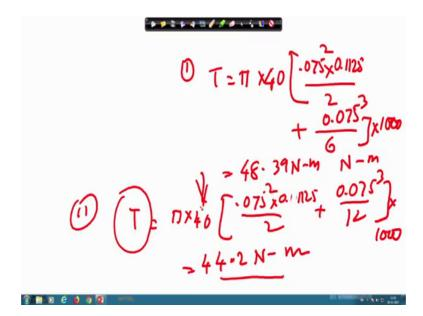
First one expression will be T will be equal to pi Cu actually forty and your it will be 0.075 square into 0.1125 divided by 2 plus 0.075 cube divide by 6 into 1000 Newton metre. So, it gives you the value equal to 48.39 Newton metre. And for second case actually it will be T equal to pi into 40 into 0.075 square into 0.0 not 0; it will be 0.1125 by 2 plus 0.075 cube by 12 here, into 1000, that gives you 44.2 Newton metre.
