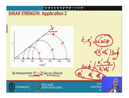
The first circle the 570, this is 600 less than that. So, sigma 1 is 570 and sigma 3 is 200. So, we know this is a 2 principal stresses. So, 2 principal stress will be on the x axis and distance between these 2 are actually the radius, diameter of the circle. So, considering this as diameter, that means I can find out midpoint and complete this circle.
