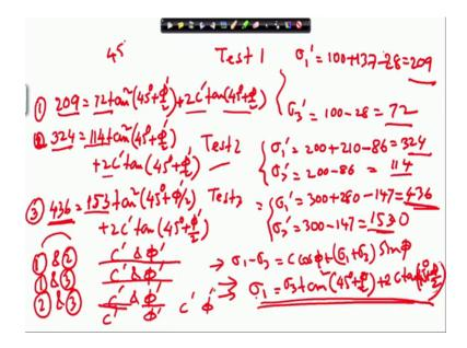
Suppose test 1, sigma 1 dash equal to 100 plus 137, 100 plus 137, it will be equal to this is minus 18, minus 228 this gives you 209 and sigma 3 dash will be equal to 100 minus 28 that is equal to 72.
