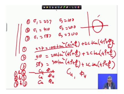
Sigma 1 was 237 and sigma 3 was 100. So, suppose from 2, sigma 1 was 410 and sigma 3 was 200 and from test 3 it was 583, sigma 1 was 583 and sigma 3 was 300. So, I can get one equation; that means sigma 3, 237 equal to sigma 1, 100 tan square 45 degrees plus phi by 2 plus 2 c tan 45 degrees plus phi by 2, phi by 2. Then from test 2, I can get 410 equal to 200 tan square 45 degrees plus phi by 2 plus 2 c tan 45 degrees plus phi by 2.
