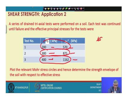
There was a test, a series of drained tri-axial test, drained tri-axial test means what? Actually this is consolidated drain. So, when it is mentioned drain test, it means it is the consolidated drain because without consolidation draining we do not do. So, that is drain test means it is a consolidated drained, automatically it is understood.
