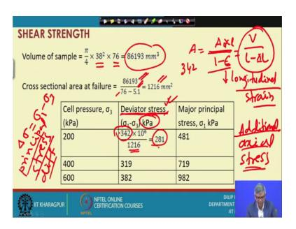
So, this is the 86193 millimetre cube and cross sectional area at failure will be suppose we have given area cross sectional area at any time will be A naught 1 minus epsilon. So, this is the, this epsilon is nothing, but longitudinal strain.
