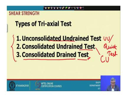
And these 3 categories namely are unconsolidated undrained test, and consolidated undrained test, and consolidated drained test and; what is the meaning of it. This is unconsolidated undrained test; that means, whatever I have already mentioned under triaxial test that we set a sample and then put a cell and then we puts water to enter with some pressure that is we by that we apply a confining pressure and then we apply axial load to shear that.
