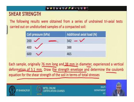
The first application is like this, you can see the following results where obtained from a series of undrained triaxial test carried out on undisturbed samples of compacted soil and we have applied different self pressures about 200 and 400 and 600 one 400 say pressure is applied additional axial load was 342 Newton. So, generally we apply we measure load and from the load we can calculate what is the stress, that actually load by area that
