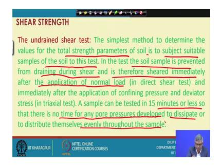
And you can see the first of all undrained test; undrained shear test, as already we have mentioned this I have before. The simplest method to determine the values for the total strength parameter of soil is to subject suitable samples of the soil to this test. That means under this test; shall we can get the total stress parameter, because we are neither consolidating nor dissipating the pore pressure.
