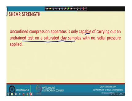
And unconfined compressive test as I have mentioned that unconfined compression apparatus that is which is a special form of Tri-axial test, where with no confinement will be there and that will be capable of carrying undrained test, the strength of the saturated
