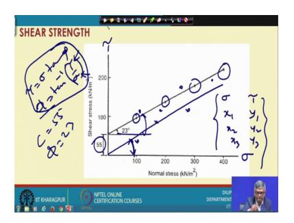
So, let us see if I take this data in a tau sigma plot, this is suppose sigma, this is sigma and this is tau and this is suppose first point 198, this is second point 200 and something, corresponding value this is about 300 and corresponding shear stress 400 shear value and corresponding as 400 normal and corresponding shear value.
