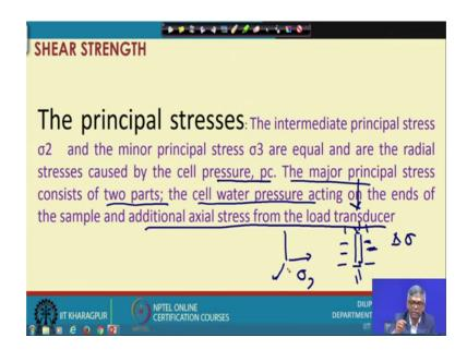
And the principal stress is you can see now I already, I have mentioned that since, we are considering cylindrical sample and then 2 though we have 3, 1, 2 and 3 direction and since it is cylindrical the 2 and 3 will be identical and they are called intermediate or minor principal stress and which is nothing, but whatever through self pressure we are applying sigma 3.
