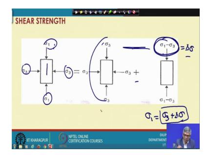
You can see that at any stage of test. So, this is the sample and I can visualize that sigma 1 is acting, sigma 3 acting and sigma 3 sigma 1 are acting. So, this is of course, all around sigma 3 and sigma 1 this is the visualization I can do for the sample.
