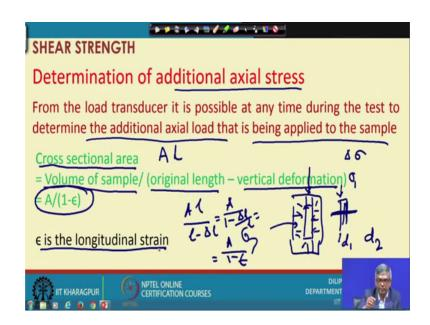
And now, determination of additional axial stress; that means, when we apply the self pressure that self pressure will be acting from all direction equally, even from the top suppose this is the sample when this is the sample and this is the chamber suppose and if I give pressure suppose sigma 3 here. So, sigma 3 will be acting all direction. So, all directions sigma 3 is there and additionally, we are giving some axial load. So, that is what is called additional axial stress.
