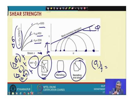
And during test actually, well different application of different normal stress, suppose sigma 3 gets 200, 400, 600, and then under different confining pressure I can apply sigma 1, minus sigma that is del sigma that is additional axial stress whatever we are applying, verses strain then we get different type of stress curve and from this I can find out what is the delta f, delta sigma at failure that mean delta sigma at failure, from there actually sigma 3 is constant.
