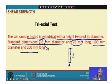
And now, Tri-axial test and Tri-axial test actually, it is the soil sample tested cylindrical samples cylindrical sample with a height twice of its diameter the soil sample tested is cylindrical; that means, cylindrical surveillance, there will be definite diameter and length if it is d and if it is l and you can see that standard, if you test on different sample will get different results.
