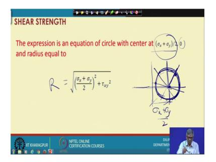
You can see the expression is equation of a circle with centre at sigma x plus sigma y by 2 and 0. So, this is x coordinate and 0 so; that means, if this is one. So, what is the centre sigma x plus sigma y by 2 and 0; that means, on this axis only the centre will be on this axis and what is this distance this is actually sigma x plus sigma y by 2.
