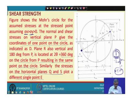
And you can see Mohr circle for the assumed stress at the stress point assuming sigma x was the bigger one than the sigma y. So, based on that we consider major and minor there are big and then 0. So, both sigma x and sigma x value are there in the plane element and they are greater than 0, but sigma is again greater than sigma y.
