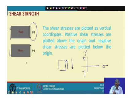
And I have to follow some sin convention actually as I have mentioned that tensile stress is positive and compressive is negative in general in mechanics, but in soil mechanics since compressive force is most important because comes there. So, compressive is taken positive and tensile is taken negative.
