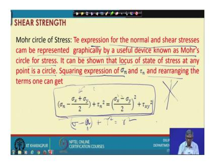
Mohr's circle of stress, the expression for the normal and shear stress can be represented graphically by useful device known as Mohr's circle of stress. It can be shown that locus state of stress at any point is a circle, that what I have shown this point, I take this direction, now I take this direction, now I take this direction, different direction I orienting the plane and then I am finding out the sigma x and tau x then that can be shown that.
