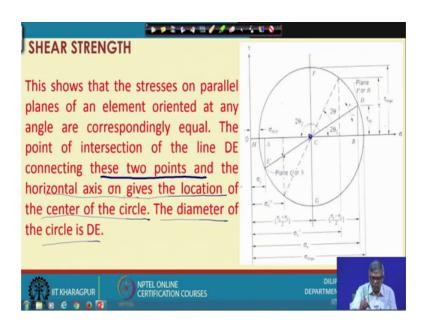
So, next slide I can show you that and this shows that the stresses on parallel planes of an element oriented at an angle are correspondingly equal the point of intersection of the line DE connecting these 2 points that means, D and E connecting these 2 points and the horizontal axis sigma n gives the location of the centre of the circle. So, this, these and
