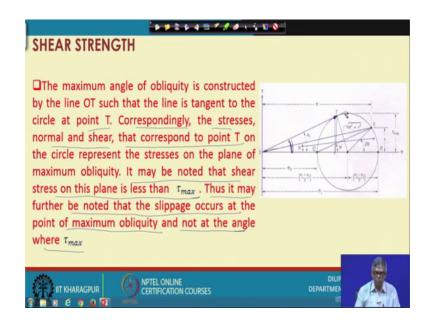
The maximum angle of obliquity is constructed by the line OT that means, you can see similar thing I have drawn here you can see here this line from point O, I can imagine number of line a one line I can dig here this line actually I can change and then finally, it will become tangent at this point suppose at point t it becoming tangent.
