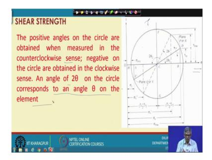
So, now I can show you that this is the Mohr circle, this is sigma direction and this is tau direction and number of things can be shown here you can see the positive angles on the circle are obtained when the measured in the counter clockwise sense that is also another important thing when the plane is rotating counter clockwise that theta is taken as positive and if it is in the clockwise direction that theta will be taken as negative.
