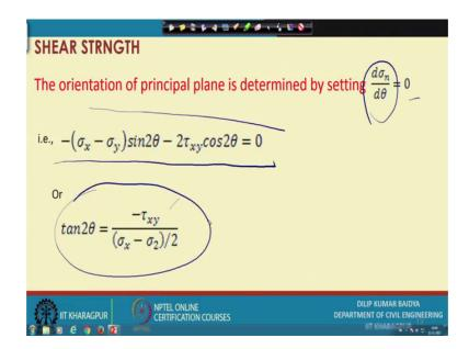
So, like this. So, the orientation of the principal plane is can be determined; that means, I have got now principal stress and we have got shear stress, and that principal stress is the function of theta with the change of theta shear stress actually changing. So, there will be definitely there is a plane, where the shear stress normal stress will be maximum.
