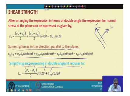
Similarly, this one if I arrange trigonometrically and we can put in a better form with double angle, sigma n become and I mean normal to that plane the sigma x plus sigma y two these are the known already, these all are known and theta also known. So, I can find out what is the value of sigma n.
