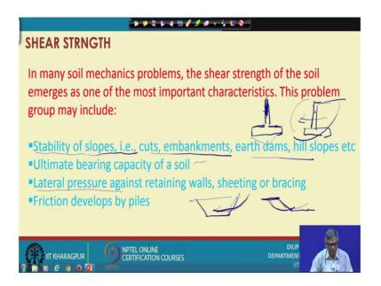
So, let me see this one shear strength, here in many soil mechanics problem shear strength of the soil emerges as one of the most important characteristics, why it is so? And this problem will be I can give you example where there important, there are several
