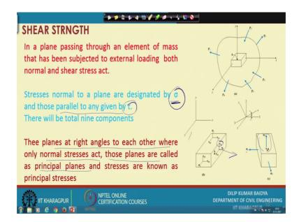
Now, again we will try to understand when the soil mass is there, and I will try to see a point in inside the soil mass, and at that point there will be number of stresses will be acting. Suppose I will take this is the one the point inside a ground mass, and which will be shown slightly enlarged view, and this is the mass entire mass and subjected to a number of forces here, and the body is in equilibrium.
