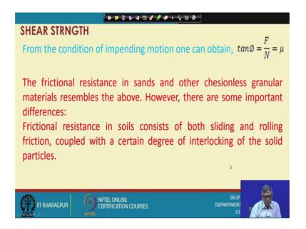
Now from the condition of impending motion one can obtain, this is the one. So, now, you know the F equal to N tan phi or mu n F equal to mu N and that is nothing, but tan phi and so, this is the relation. So, tan phi I can obtain by this tan phi equal to F by N; that means, what is the frictional resistance and what is the normal that ratio will give you the tan phi
