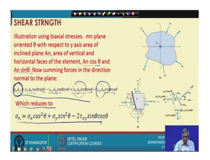
Now, illustration using biaxial stress; that means, whatever we have done that is actually three dimensional some time is not essential always to use three dimensional, most of the soil mechanics problem can be used in by two dimensional, and we cannot try to understand that. So, similar figure I have shown the body, and similar one point I have
