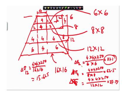
This is the 4 meter footing and suppose different depths 2 meter, that is suppose 4 meter and this is suppose 8 meter and this is suppose 12 meter.
