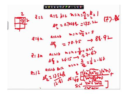
So, it will be 2 by 2 and here actually z actually suppose 2 meter first and here if I consider this small one then it will be a equal to 2, b equal to 2. So, m equal to a by 2 equal to b by 2 nothing, but it will be 1.
