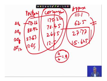
Point load delta sigma z 2, delta sigma z 4, delta sigma z 8, delta sigma z 12 by point load we have got 173.26, then we have got 88.92, then we have got 27.63, then we have got 12.81.
