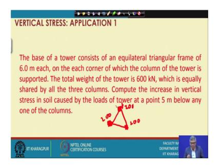
So, 1 problem is this, first problem was, is like this the base of a tower consists of an equilateral triangle frame of 6 meter each. On the each corner of which the column of the tower is supported the total weight of the tower is 600 kilo newton which is equally
