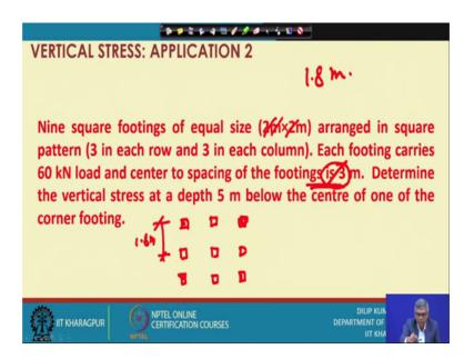
So, this is the first application and second one 9 square footings of equal size that is 2 meter by 2 meter.
