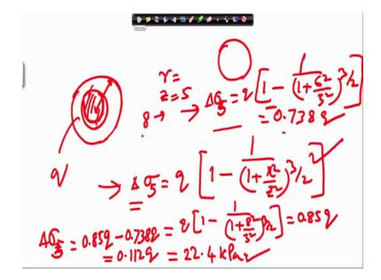
This actually I can do by applying method of superposition and you can see it is given radius of 8 meter with outer radius and 6 meter. So, this is suppose 8 meter. And suppose I assume this entire area is loaded with intensity q then at 5 meter depth delta sigma 5 I can find out there is a by integration for circular footing at the centre we have done q multiplied by 1 minus 1 by 1 plus r square by z square to the power 3 by 2.
