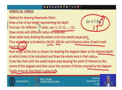
You can see here method for drawing new marks chart, first thing is you have to draw a line of any length representing the depth that is suppose 2 centimeter line suppose I have to do, I have to draw the chart how to fix the length in such a way suppose I only use a 4 size paper, so 9 circles at least it should come within the paper. So, 2 centimeter 3 centimeter anything can be taken and that should be that line also drawn at the side because that is the scale used for drawing the in pressure.
