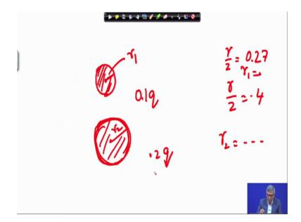
Suppose 2 values r by z equal to if I go back r by z is 0.27 and 0.4 suppose r by z 0.27 and r by z equal to 0.4. Now if I fix the depth equal to z 2 meter then r will be some value suppose that is suppose r1; that means, if the circular loaded area is r1 something with radius r 1 and that much load area if loaded with intensity q at 2 meter depth your intensity will be 0.1q. Similarly now if I now do r by z equal to z is the same now if I do same then 0.4 this is the 0.4.
