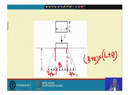
So, this is actually has have told 1 vertical n horizontal here actually 2 horizontal 1 vertical a 2 vertical 1 horizontal this is a standard thing we use, and if you use this then this become B and this become z by 2 z by 2. So, ultimately this width becomes B plus Z. So, if is a rectangular footing B plus Z will be width and say length also will become L plus Z, so at this depth area will be this multiplied by this.
