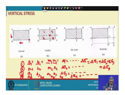
You can see here whatever derivation we have done this is suppose the typical foundation and with dimension is a and b, this is get application of whatever formula we have given. So, we can consider this as a and this as b and at this point suppose we want to find out the stress. So, directly we are applying the corner formula, but if instead of at this corner if I want to find out the stress at some other point suppose at the interior of this point of this foundation.
