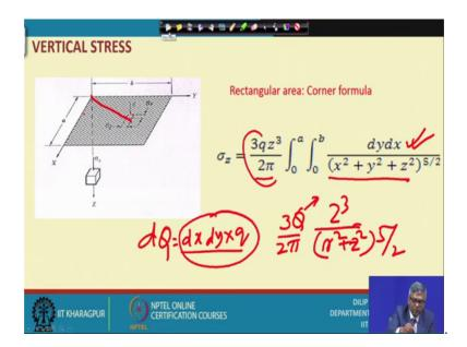
Suppose the rectangle with size a and b and then in that case how to do this integration you can see here this is a x axis from x axis at a distance suppose dy at a distance at a distance y at a distance y I have taken a small width dy and from x y axis at a distance x I have taken dx width.
