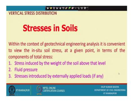
And now this is actually a stress in soils in general with within the soil. In the context of geotechnical engineering analysis we can divide into 3 important parts, one is stress induced by the weight of the soil above that level; that means, soil may be considered at a depth of 5 meter. But, above the above the 5 meter or entire depth of the soil, there will be weight and that because of that weight at 5-meter depth there will be some stress.
