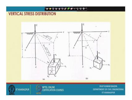
We are as user will be using the boussinesq theory and here actually initially when it is develop the boussinesq theory, it was actually in the rectangular coordinate system XY and we can consider at a point X which is sorry point any point at a depth Z. Which is at a distance X from the Y it is axis, Y from the X axis and at Z from the XY, XY plane.
