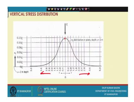
This is one observation second observation is when we are we suppose if Z is fixed; that means, I want to find out at a point load is applied at the surface, but I want to find out a 2-meter depth and from any distance from the point of application of the load. Both side if I go.
