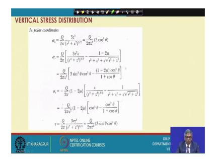
This is actually sigma Z that in terms of theta shown in the previous figure. Similarly, sigma R; that means, radial direction there is a component sigma T there is a tangential that is a component and there is a tau. All those stress components are there.
