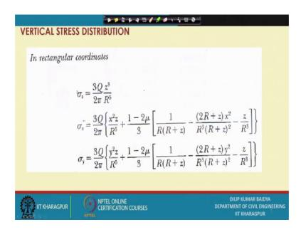
Here this is given sigma Z expression 3Q by 2 pi ZQ by R to the power 5 this R is what actually here it is shown you can see this is the R this is the R. You can find out this small R as under root excess over X square Z square and this is again Z. This R square plus this Z square ultimately will be under root X square plus Y square plus Z square.
