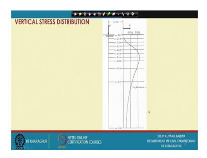
Now, As 2 variables are there one is R another is Z and because of that you can see here if I fix the value of R that at a particular distance of load is applied here and I have taken at a some distance about 2 meter and then I very Z then over the depth how this vertical stress is varying?
