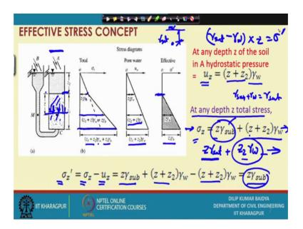
So, suppose this is a situation here and you can see that this is a soil, mass this is a soil mass and it is a through this soil and water head is applied here and from the bottom also it is connected to another tank and the water is continuous through this end to this end A to B. But since there is a overflow from both places if there is a water more either here or here it overflow will take place and maintain same level..
