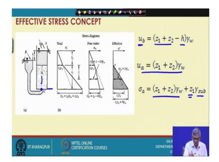
So, you can see that this is the one as I have mentioned there that I have considered a tank is a lower height and we are supplying flow here at a particular height and the difference is h. So, because of these changes, change in head at this side and at this side then; obviously, flow will take place in this direction.
