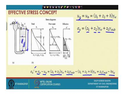
Now, there is a third case we will consider that is actually as I have shown before that the third condition whatever I have shown that when this tank is elevated or lifted some by some height and you can see here and this is the level here and this is the level here. Now, if I continuously supply water here and then because of this the water is continuous throughout this then this water will try to flow through this soil in the upward direction.
