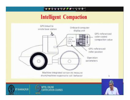
There is nowadays, we have intelligent compaction that intelligent compaction means that equipment is (Refer Time: 26:39) by itself will have some various accessories which
