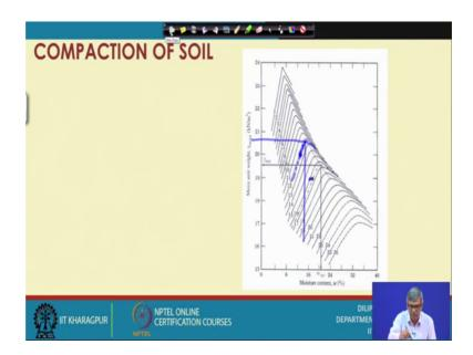
This is another of course, we are going to have different energy level curve here and from there actually again, we can put our uh obtained 1 point from here, from here; obviously, we can they are all very close lines. So, automatically the curve will fall somewhere here. So, from here also one can find out optimum (Refer time: 18:46)
