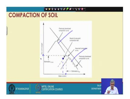
Similarly here, sometime we have some compaction curve of different energy level and suppose by 1 point method also sometime we can find out, what will be the optimum moisture contents. If I use I have suppose a curve with 1 energy level, I have another energy curve with another energy level; but I neither use this energy neither nor use this energy.
