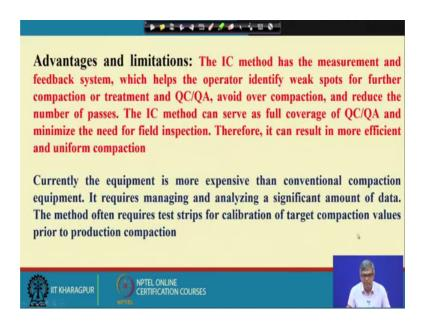
And advantage will be you can see the IC that means, Intelligent Compaction method has the measurement and feedback system which helps operator identify weak spots for further compaction or treatment and Quality Control or Quality Assurance avoid over compaction, and reduce the number of passes. So, suppose though we have recommended 6 passes for a particular dry density, but if I find that the 4 passes we are achieving that. Then, we can stop that is the advantage.
