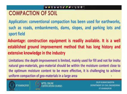
And this is compaction, conventional compaction actually is used for earthworks, the road, embankments, dams, slopes, parking lots and sports field. These are the areas actually commonly that type of compaction equipment; I have mentioned they are used for this type of work mostly. And it has some advantages and it has some disadvantages. What are the advantages?
