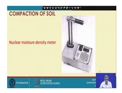
Nuclear moisture density meter; like that. In the field directly we can get moisture and density and how this it work actually? The Apparatus is placed, Apparatus placed on the ground or compacted fill and emits gamma rays through the soil. Some of the gamma will be absorbed other will reach to a detector. And Soil unit weight is inversely proportional to the amount of radiation that reaches the detector. So, that is the way it works and it also can sometime measure the moisture.
