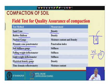
So, for that actually, there are number of methods are there Sand Cone method. There is a method called Sand Cone method. Then that to find out density the Rubber Balloon, Nuclear Gauge, Dynamic cone penetrometer, Soil stiffness gauge. There are so many equipment nowadays available, but typically most easy way, easy easiest way actually what we can do that sand replacement method.
