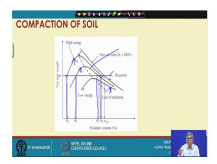
And then, another thing is as I have mentioned that when we change the level of energy then, automatically what happens? Your compaction curve shifting lift left and with higher dry density like you have 1 compaction curve for a particular soil, with this much energy the another is second level of energy; there is another third level of energy.
