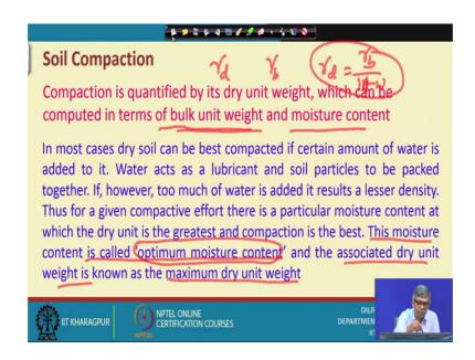
Compaction is quantified by it is dry unit weight which can be computed in terms of bulk unit weight and moisture content. We have actually at the beginning we have done so many things. Actually, we have done gamma d, we have done gamma bulk and we have got the expression relationship become gamma d and gamma b relation is 1 plus w. This is done at the beginning. That is what?
