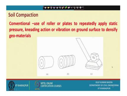
So, soil compaction typically we do by using different things. This is a roller. This is also sometime rubber tire roller. This is smooth wheel roller and this may be sometime plate compactor. So, different way on the soil we put a layer of soil and then we can by some way you can apply over a dense.
