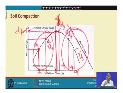
And this is actually to test soil, if soil is tested in the laboratory and then generally we get a compaction curve. So, as I have mentioned that we have to see we cannot add water excessively. You have to do travels actually initially. We have to start with some minimum level of water content 4 to 6 percent and you have to compact the compaction; that is a standard procedure.
