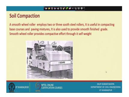
And now the soil compaction. I have several things I will discuss, but during for compaction, generally different types of compaction is used. There is a smooth wheel roller of compaction. The smooth wheel roller employs 2 or 3 smooth wheel rollers. It is useful to compacting base courses and paving mixtures.
