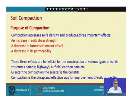
So, now Soil Compaction; what is the purpose? Purpose of compaction is compaction increases soils density and from immediate effect what do you get? The soil particles comes closer and density get increased and that actually gives you several benefits and that is most important 3 are actually increase in shear strength and decrease in settlement. That will compressibility and decrease in permeability.
