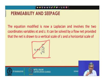
So, now the equation modified is now Laplacian and involves the 2 coordinates variables. One is x t and z. Originally it was x and z. Now it become x t and z. It can be solved by a flow net provided that the net is drawn to a vertical scale of z and a horizontal scale of x t equal to this. So, this is the change actually. The horizontal k scale
