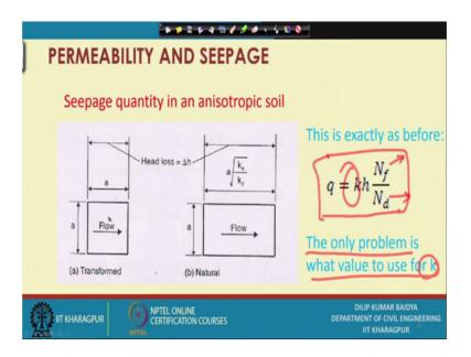
I have taken now the 2 sections. This was the natural section. Suppose x equal to. This is x actually. This is the x and maybe some relation it is there and this is y direction is a. And this transformed a in this form and in this transformed when we were transforming this the same equation is valid; that means, this is exactly as before; that means, I can use this equation q equal to k into h into N f by N d. Then once you draw the transform section below the structure.
