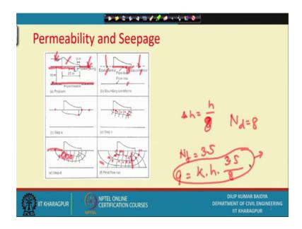
We have mentioned that we can try to make while drawing the flow net, we will try to make equally square blocks. The size will not be the equal. All block will not be equal size.
