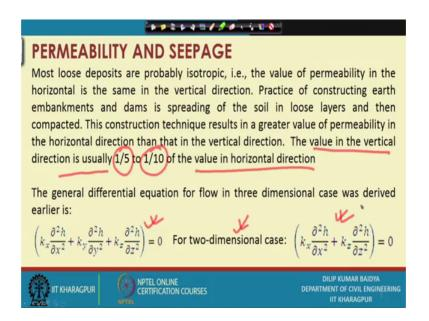
So, now most loose deposits are probably isotropic; that means, if the soil is loose condition, then when flow take place, then flow all direction will be almost equal value; that means, value of permeability in horizontal is the same is in the vertical direction, but actually in the practice when there will be this type of structure is constructed, generally it will fill in layer and then it will be compacted.
