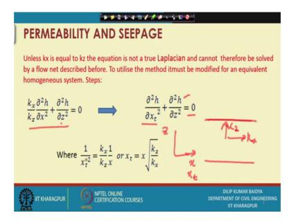
Now, unless k x as I have mentioned that unless k x is equal to k z. That the equation is not true Laplacian equation and therefore, be solved by a flow net described before. To utilize the method, it must be modified for an equivalent homogeneous system; that means, when k x and k y is different and suppose this the soil mass and the k x value is this k z, this is k x and this is k z and if they are different then I cannot apply that.
