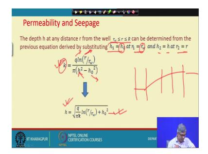
And next slide, actually sometime we need to find out what is the, at a distance, at a distance of x, what the water height, because sometime we have to find out (Refer Time: 13:30) because excavation area sometime, is a large. Suppose in a particular point we are doing this, but at a distance from this construction site, what is the water height that to be determined. For that actually we can do this way h 1 equal to r naught at r 1 equal to rw, and h 2 equal to r and r 2 equal to r
