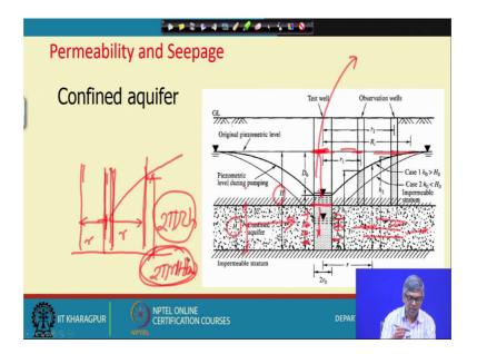
Next slide is, actually as I have told you, that water bearing layer can be unconfined or confined. This is a case of confined aquifer. This is a confined aquifer, and this confined aquifer, actually confined means what actually here. You can see it is same as previous. Only thing, this is actually maybe very thick clay layer and this is impermeable layer, this is impairment layer. This is the layer sand which holding the water.
