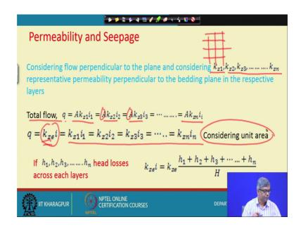
Now, the other case, when the flow is taking place, perpendicular to the bedding plane. Considering flow perpendicular to the bedding plane, and like kz the 1 kz 2 like that respective permeability value in the layers, and kze. Maybe I can take consider as a
