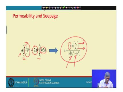
So, if I put in the integral form. So, it comes like this. You can. Since we have two observation well r 1 r 2, I can put limit r 1 to r 2, and q also I can put q already is there 1 by r del r, this is actually variable. And 2 pi k is I said I can keep constant and h del h is the variable. So, I put this and limit h 1 and h 2, and if I integrate and simplify, then I will get finally, equation for k q ln r 2 by r 1 pi h 2 square minus h 1 square. So, this is the one equation
