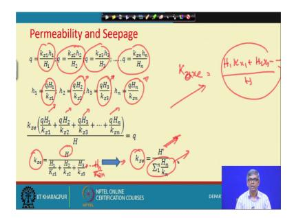
Now, q equal to I can express in this form, q I can express, I can express in this form. Again q I can express in this form, I can q also can express. Everywhere q is same for different (Refer Time: 30:35). So, H 1 I can calculate this way, H 2 I can calculate from this way, H 3 I can calculate this way. So, because q value are same, then I can find out this.
