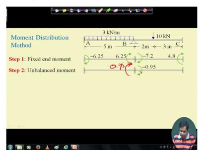
Now these unbalanced moment needs to be met 0, right because there is no externally concentrated moment here, so moment and B both the segment they should cancel each other. Now next it is we have to make it 0, how do I make it 0? Just by if we apply and if it is minus point if we apply an additional moment here which is 0.95 suppose fictitious, you apply an additional moment which will balance each other, right. Now then this equilibrium is satisfied, we are going to do that.
