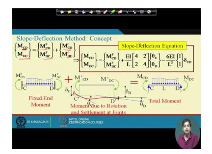
Now, so, now we have determined, we have seen how to determine the fixed end moments and just now we have seen how to determine this. So we have this with us and we have this with us. Then this + this is equal to this, though M CD will be, so M CD will be, M CD will be M dash CD + M fixed end moment CD. And similarly MDC will be this + this, right. So then what we have is, if we write that again in a matrix form, say M CD will be, M CD will be this + this and M DC will be this + this, okay.
