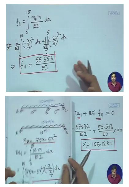
Now what is the value of F 11, S 11 will be 0 to 15 because this is the total length, then m1 into, in this case there is no m1 because there is just only one redundant force, so it is m into m by EI dx. Okay. And the expression for m, we know that this becomes 0 to 10, X is - X by 3 whole square dx 1 by EI and is equal to + 0 to 5, it is again -2 by DX 1 by EI, 1 by EI, okay. And this becomes, F11, if you do this integration and this becomes 55.556 divided by EI, okay.
