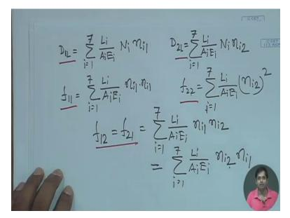
Now we know that D1 L is equal to how to determine that, D1 L is equal to summation of i is equal to 1 to 7 here because we are 7 members that is then Li by AiEi into Ni and since it displacement in the direction of first redundant this will be ni 1, okay. And similarly D1 L, similarly D2 L will be summation of i is equal to 1 to 7 Li by AiEi and then Ni and it will be ni 2 due to second redundant, okay.
