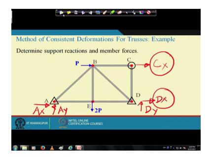
So let us take this problem this is again an indeterminate truss, okay so first thing is we need to find out what is the static indeterminacy you see here number of members are 1, 2, 3, 4, 5, 6, 7 so M is 7 and number of joints are 1, 2, 3, 4, 5 so J is equal to 5 and r is equal to here you have 2 reactions two reactions 4 reactions and then we have 1 reactions here so total 5 reactions.
