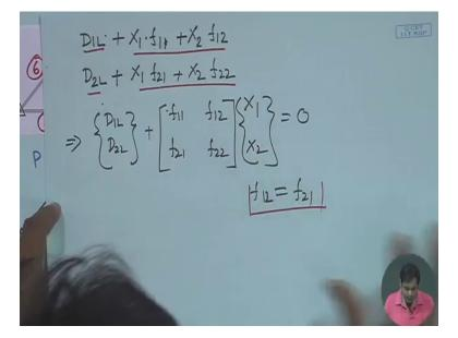
Now suppose okay, now we have so we have 2 joints 2 redundant forces here, X1 and X2, X1 is at point C, X2 at point D so we need to consider the displacement at point C and displacement at point D, okay horizontal displacement at point C and horizontal displacement at point D.
