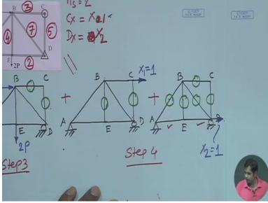
Now once we know these are 0 force member and it is a statically determinate truss we can compute the forces in other members and if we do that I have the force ready with me this is written as ni small ni and then write 1, 1 because it is due to the redundant force 1, okay whose value is X1, but it is obtained these values are obtained when the unit load is applied in the direction of X1, okay.
