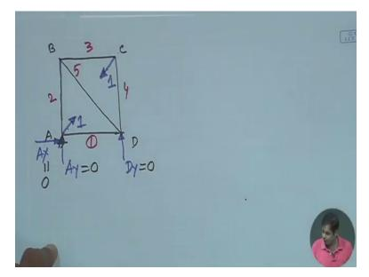
That is what unit load method we discussed some time back, so we apply an unit load here. So let us find out what is the corresponding member forces, so draw the structure once again free body diagram of the structure, so this is the truss and then this is A, B, C, D another member here member AC, then what are the forces we have? We have Ay, then Ax and then Dy and then unit load here unit load 1 here, okay and then member force member numbers are 1, 2, 3, 4, 5 and this one is 6, okay.
