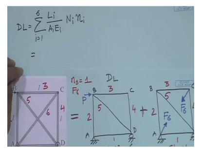
We can apply unit load method DL if we apply unit load method then DL will be the unit load method is in the direction wherever you want to determine the deflection we apply unit load in that direction and then analyze it and then once we get the results then DL can be obtained as for truss summation of i is equal to 1 to 6 in this case because there are 6 members and then Li divided by Ai Ei into Ni and small ni, okay.
