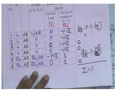
So let us do that, so if we do that then this becomes L by AE this is L by AE, right? The length is L by AE into this P into minus 1 by root 2, right? And then this also same this is also same this is 0, this is also 0, this is also 0 and this becomes root 2 L by AE into minus P by root 2, okay. Now so then what we have is P by root 2, P into root 2 sorry P into root 2, okay.
