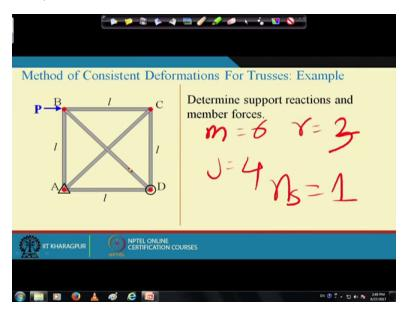
So let us take this is our second example this is again a statically indeterminate truss you number of total member is total member if you take in this case total member m is 1, 2, 3, 4, 5, 6 m is 6 and r is equal to 2 r is equal to 3 two reactions at A and one reaction at D and number of joints is equal to 4 so total number of equations available 4 into 2 8 and the number of unknowns are 6 plus 3 9.
