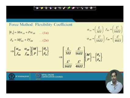
Now then what we have is equation number 1 a is this and equation number 2 a is this and in this equation alpha and F they are the flexibility coefficient associated flexibility coefficient that expressions are this, ok.
