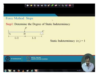
So let us summarize the different steps that involved in force method and the steps are let us take this example the same example that we that we analyze in the last class. The first step is to once we have any statically indeterminate structure and we need to solve it using force method.
