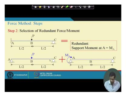
Then step 2 is now once we know the static indeterminacy then we need to select we need to choose the redundant force or redundant moment. For instance in this case static indeterminacy is 1 so we need to find out what is the redundant force or what is the redundant moment, ok.
