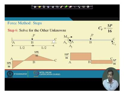
Now once we know C then how many it is a free body diagram of the entire structure this is the last step, you see here 3 reactions at A and 1 reaction C y. There are 4 reactions we could not solve using equilibrium equation. Now we have already determined what is the value of c y using the compatibility at compatibility condition at C.
