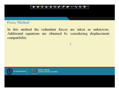
So what we have seen in the last class is force method is in force method the redundant forces are taken as unknowns, and additional equations are obtained by considering the displacement compatibility, ok.
