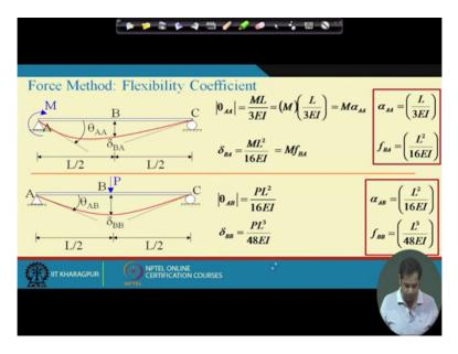
Now take one more problem take another case where the same simply supported structure, but now it is subjected to a concentrated load at the mixed span. And the red line that you can see that is the deflected shape of the beam. And these slope at theta is theta AB, and deflection at B is equal to delta BB. Slope at theta AB means it is slope at A due to force applied at B.
