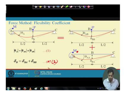
So now what we have is now suppose consider now in this problem the loads are acting separately it is only concentrated load it is only the moment at A. Now suppose we consider a problem like this where the same simply supported beam but it is subjected to both a concentrated load at the mid span and moment M at point A, ok.
