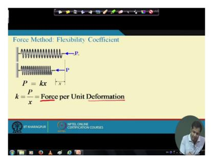
Now let us see if we have a spring which is subjected to actual load P and then because of this load P the this spring undergoes the formation and suppose this the change in length is x, ok. And then we know that P is equal to kx where k is the stiffness of this spring or sometimes it is also called spring constant.
