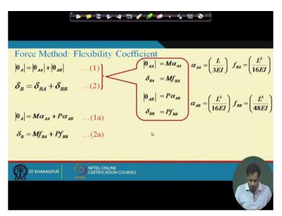
Now if we apply this into these two equations which we obtained from Principle of super position. Then what we have? We have this theta A is this theta AB is this and theta BB BA is this and theta BB is this. So we have these two equations suppose this is equation number 1 a and this is equation number 2 a, ok.
