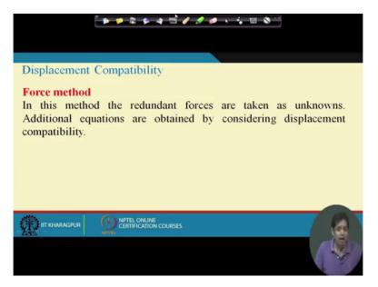
Now then we have to formally introduce force method. What is force method Force method is in this method the redundant forces are taken as unknowns and if you remember the redundant force means we for the previous problem the prop Cantilever problem we took support reactions at prop or moment at the fixed length are unknown because they are the redundant forces ok.
