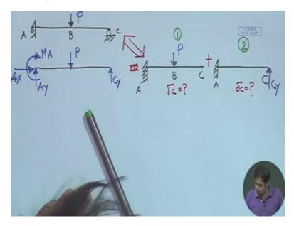
Now let us see what we can do Now the problem is like this it is a the Cantilever beam and then it is a ok then we have on externally used blue ink externally load say P here. So this is A this B and this is C. We need to find out what are the support reactions.
