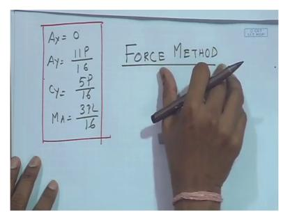
So the final solution will be for this problem is this x is equal to 0 any where x is equal to 0 A y will be is equal to 11 P by 16 C y will be 5P by 16 and M a is equal to 3 PL by 16 This is the final solution.
