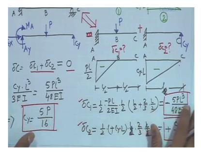
So this is force method, ok? Now in this case these what we actually did is we looked at the problem first and implicitly without actually unknowingly we determine the degree of indeterminacy in this case degree of indeterminacy is 1 and this indeterminacy external indeterminacy ok.
