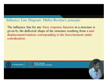
Now let me demonstrate this through one example, before that what Muller-Breslau's principle says, It says the influence line for any force response function. You please note it, force when I say force response function it could be support reaction, it could be shear force at any particular point, it could be bending moment at any particular point,
