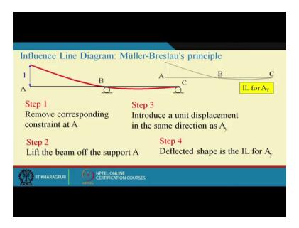
So let us see the steps then, so we have the beam here the continuous same beam, the first step is remove corresponding constraint at A, suppose we want to find out the influence line diagram for vertical reaction, so remove the corresponding constraints this is step one and then step two is lift the beam of support A.
