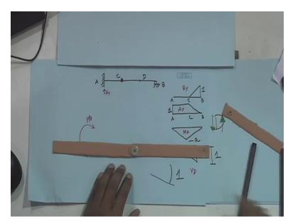
Now suppose this is the model ok. This is the beam ok, let us first draw the beam; the beam is a propped cantilever beam. We have a propped here and then in addition to that we have an internal hinge here ok and this is A, this is B, this is C and this is D, what we want is we want to find out what is the influence lien diagram at support reaction at A,
