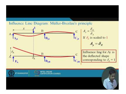
So we have let's see what it says you then A Y is equal to delta x by delta A, now this is too for any value of F A and any value of delta A right, now let the force is such that delta A is equal to one ok, so the force is the deflection at point A is reduced to one, is scale to one if we do that if delta A scale to one then what is this A Y become delta x right.
