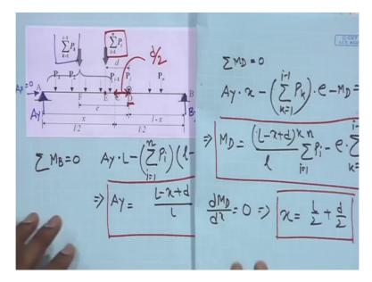
What is you see x is equal to L by 2 means at point C, ok this x. And then D by 2 means D is the distance of D from the resultant of the entire load so this distance so CD if CD if this distance becomes D by 2 then the moment at D will be maximum, ok.
