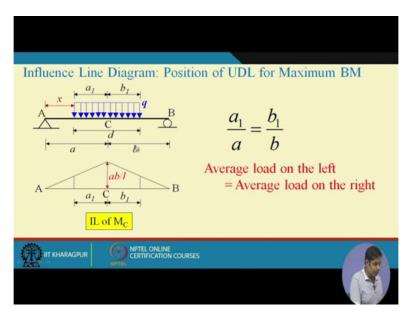
We have done it for uniformly distributed load. This is the we have already prove in the last week that if the load is uniformly distributed load and subjected on a simply supported beam because this is mean structure can be idealized in the simply supported beam.
