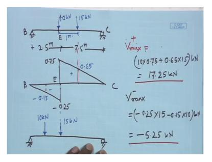
Now just quickly we will check what would be the position for maximum shear force if this is this point is E this is 2.5 meter and this is 7.5 meter we know what is the Influence Line Diagram for shear force, Influence Line Diagram for shear force is this. This value will be 0.25 or minus 0.25 and this is 0.75 this is B C B C this value is E, ok.
