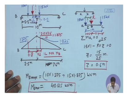
So let us try this problem so quickly it is simply supported beam and this length is total length is 10 meter, ok and then we have a point E which is 2.5 meter distance, ok. We are going to find out what is the let us first do it for maximum bending moment.
