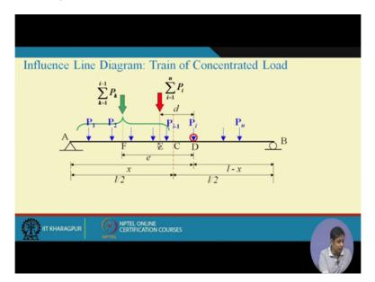
Now suppose this is a same beam AB simply supported beam and this beam is subjected to and C suppose is the center point of the mid span of the beam. And so if the total length L so AC is L by 2 and CB is L by 2 ok. Now suppose this is subjected to a train of concentrated load. And this distances between two consecutive concentrated loads are same not same they remain same they do not change as the load moves on AB, ok.
