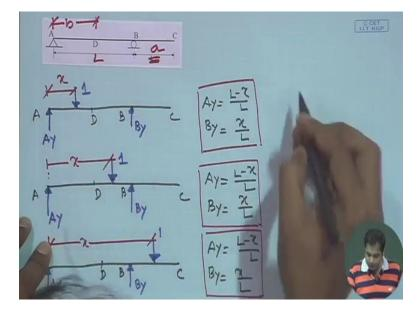
And the reactions will be in this case A Y is equal to L minus x by L and B Y will be x by L, in this case A Y will be L minus x by L and B Y will x by L and the third case it is A Y will be L minus x by L and B Y is x by L, so what we can see is, in all the cases support reactions are same ok, please verify this ok, these are all support reactions ok, now we need to find out what is the bending moment and shear force at point D.
