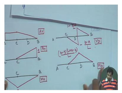
Now similarly if you draw the shear force bending moment diagram between A and C it is zero, just now we check and then it becomes this value. And this is A C D and B this value is B minus A into L plus A minus B by L, this is for bending moment at D,
