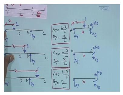
So if we take the free body diagram of this part so we have A Y and at D we have B D and moment M D and unit load is one at a distance x ok, and this distance is B ok, now similarly if we for this case take the free body diagram of same part this, the free body diagram will be, there is no unit load here it is just only A Y and then V D, M D there will be no load because load is now D B, this is A and D, A D A D ok and third case also same thing.
