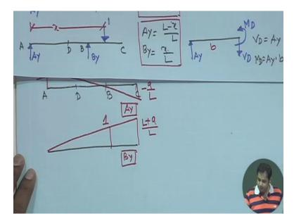
Now let us draw influence for B Y, what is B Y, B Y is x by L here, x by L here, x by L here, x is equal to zero, then B Y is equal to zero, and after that this linearly varying so it varies linearly
