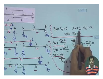
Now first draw the influence line diagram for say A Y ok, now what is expression of A Y, A Y is equal to one when for the first case when load is between A and C and then all other cases A Y is equal to this it is linearly varying ok and at x is equal to, if we substitute x is equal to (13:18 L plus A) means at B this A Y becomes zero.
