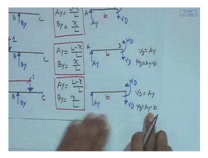
we can find out what is the expressions for M D and in this case what will be the expression for V D, in this case V D will be A Y, in this case also V D will be A Y. A Y already we obtained here, in this case also A Y we already obtained and what will be M D, M D will be A Y into B ok.
