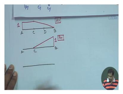
So B Y is equal to zero up to C and then at B it becomes one and between this it varies linearly, so this is one, so this is for B Y, so this is the influence line diagram for B Y, let us draw it for another support reactions means M A, this is again A C B, ok.
