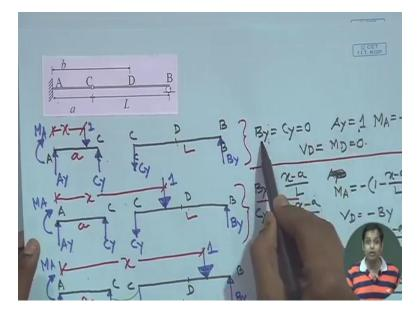
What is the value of B Y if you check, B Y is equal to zero when the load is between A and C and B Y is equal to x minus A by L when the load is between C and D and D and B both means between C and B the B Y varies. As x minus A by L, so if you substitute at x is equal to L plus A means at B, so this becomes one.
