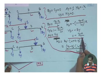
Now shear force at D when load is between A and C is equal to zero. Shear force at D varies like this when load is between C and D.
