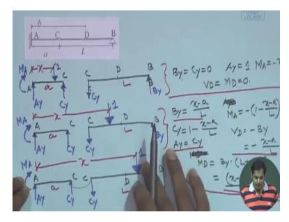
Now we can see that there are three segments AC, CD and DB, we need to consider three cases, one is influence line when the unit load is between A and C.
