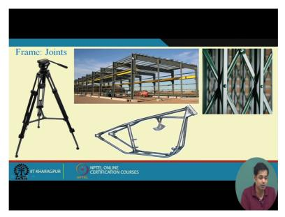
If you take a frame of a cycle, this is a frame and these joints are also rigid joints. There is no rotation allowed in these joints. This joint, this joint, all are rigid joints.
