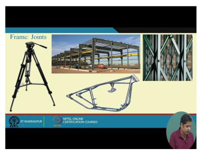
There is no rotational constraint in all these joints. But still it is not a truss, it is a frame. Why it is a frame? Because another important part in case of truss is all these members are separate members, okay. They are connected only at the end. Now here this is one member and this member is connected to this member at some intermediate point, not at the end points, okay.
